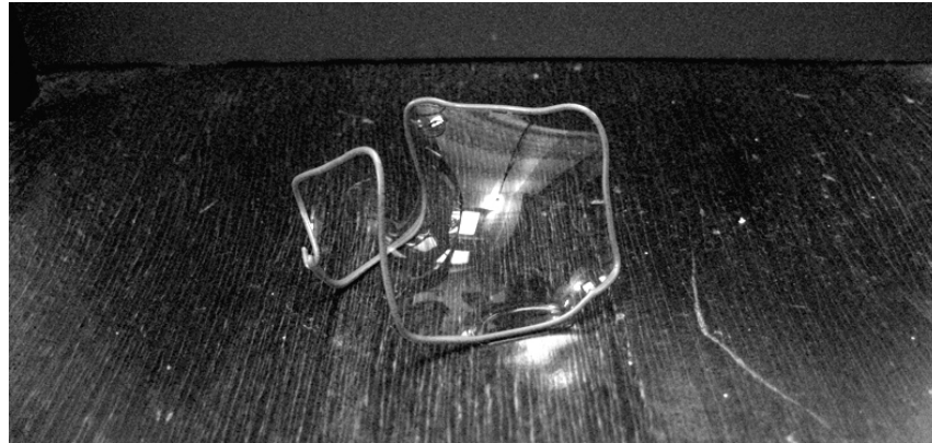
Figure 6.1: Plateau's problem for minimising a surface area involves finding a surface function. A soap film can solve the problem by assuming a surface of minimal energy
