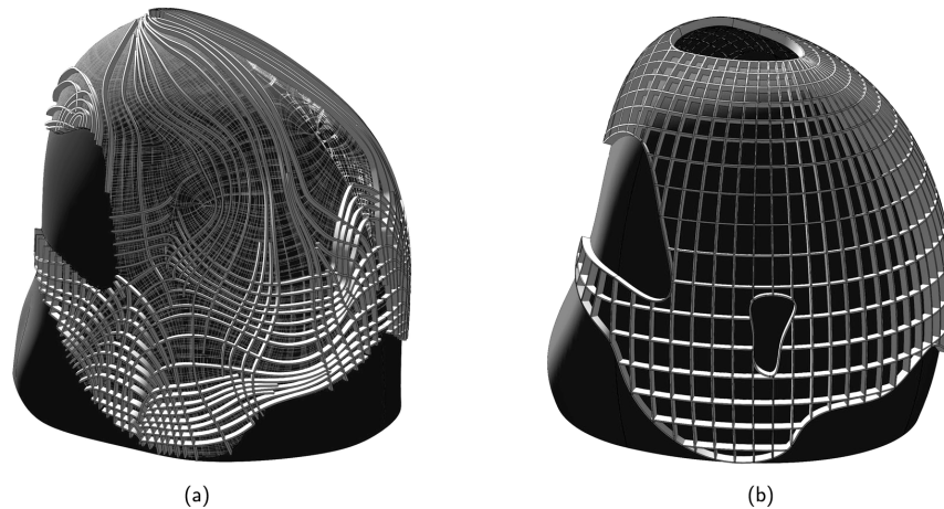
Figure 2.11: Orchid House [22Orc]. Initial torsion-free member layout (a) is rationalised through small modifications to the underlying form (b)
