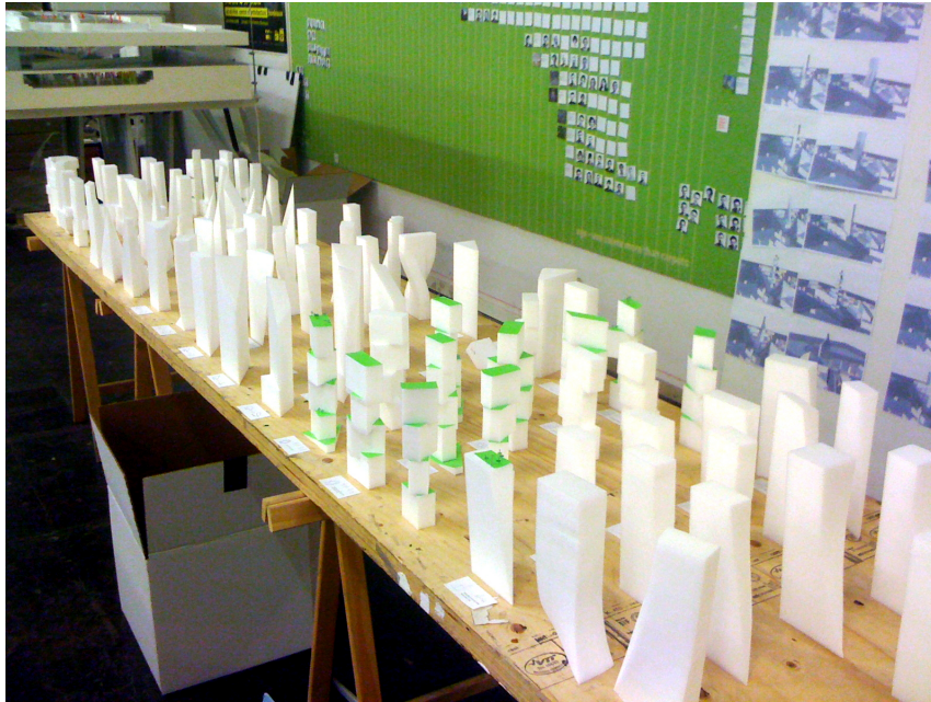
Figure 4.3: Foam models allowing exploration of different design typologies on the Escher Tower project.
