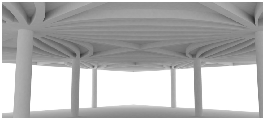
Figure B.1: Concrete slab (Viikki Synergy Building [10Vik]) with ribs aligned with principal bending stress paths
