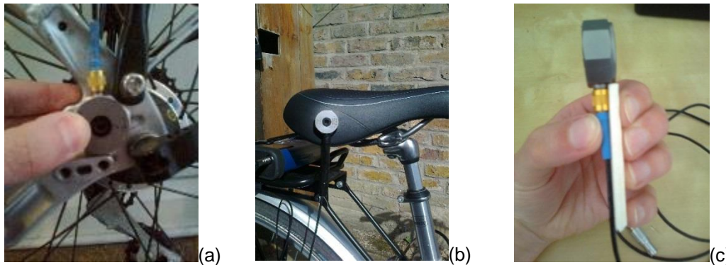
Figure 4 Fixing to frame at rear axle (a), to saddle (b) and wooden lathe supporting the cable (c)
