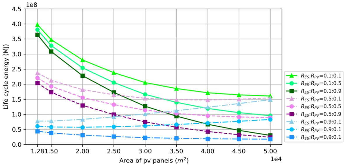
**Fig. 10.** Life-cycle energy consumption at different recycle ratios of electricity storage and PV panel.
