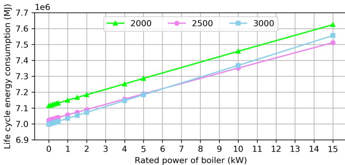
**Fig. 12.** Life cycle energy consumption at different design areas of PV panel.
