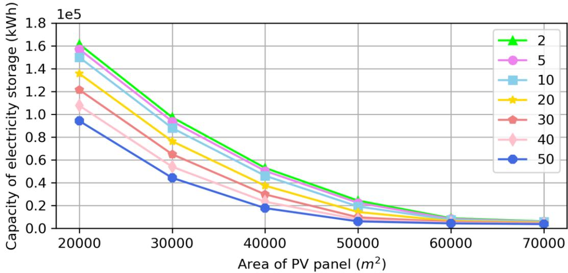
**Fig. 20.** Relationship between the capacity of electricity storage and PV panel areas at different limited electricity importation rate.
