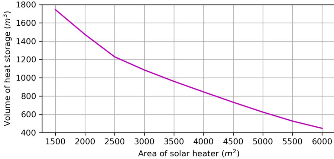
**Fig. 4.** Relationship between design capacity of heat storage and design area of solar thermal collector.
