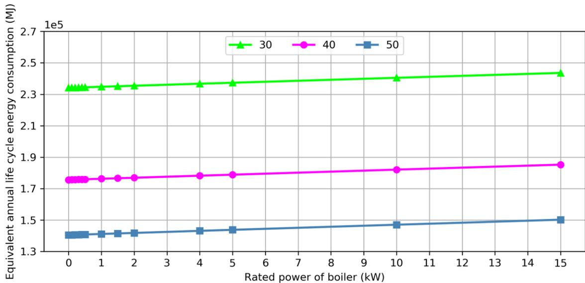
**Fig. 16.** Life cycle energy consumption at different life span.
