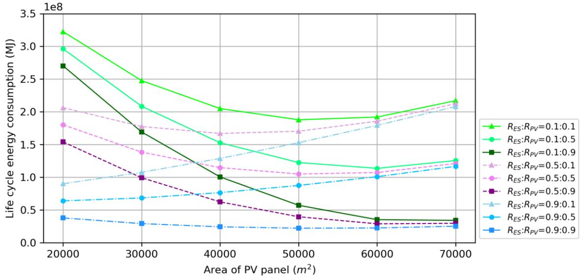
**Fig. 18.** Life cycle energy consumption at different recycle ratios of electricity storage and PV panel.
