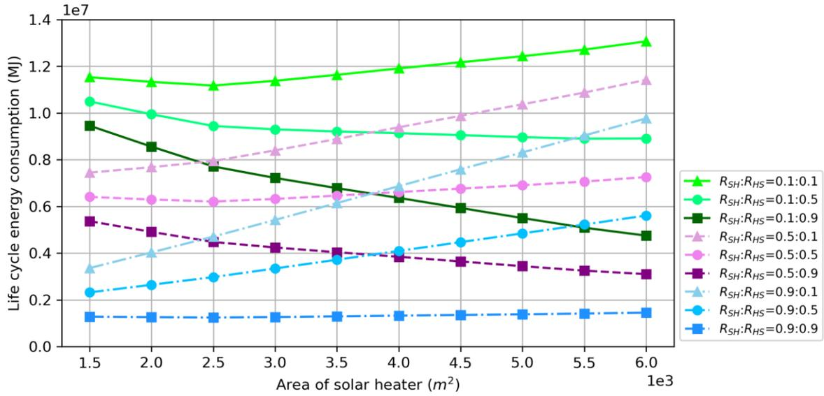
**Fig. 6.** Life cycle energy consumption at diverse recycle ratios of solar heater and heat storage.
