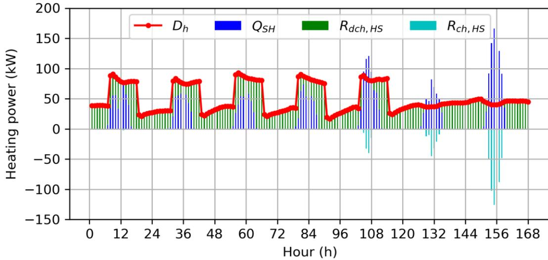
**Fig. 5.** Heat power distribution between solar thermal collector and heat storage.
