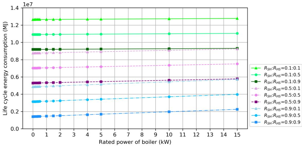
**Fig. 15.** Life cycle energy consumption at different recycle ratios of solar heater and heat storage.
