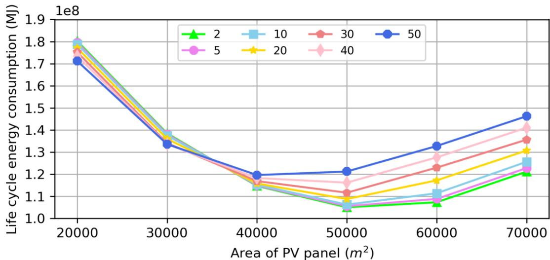
**Fig. 17.** Life cycle energy consumption at different limited electricity importation rate.
