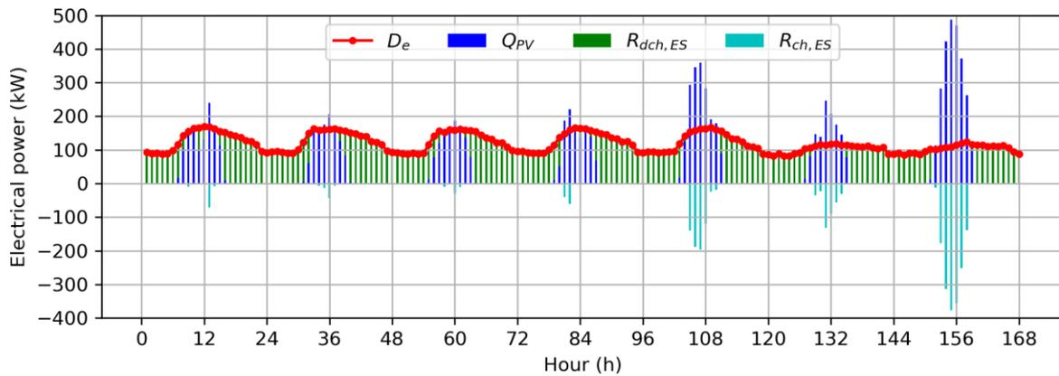
**Fig. 9.** Electrical power distribution between PV panel and electricity storage.
