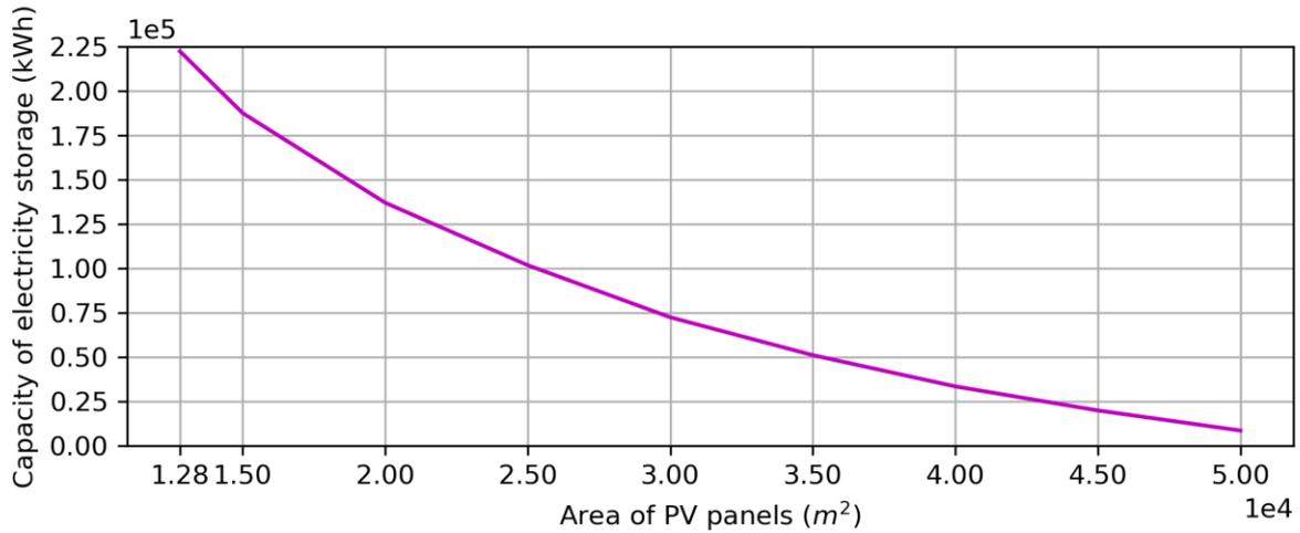
**Fig. 8.** Relationship between the design capacity of electricity storage and design area of PV panel.
