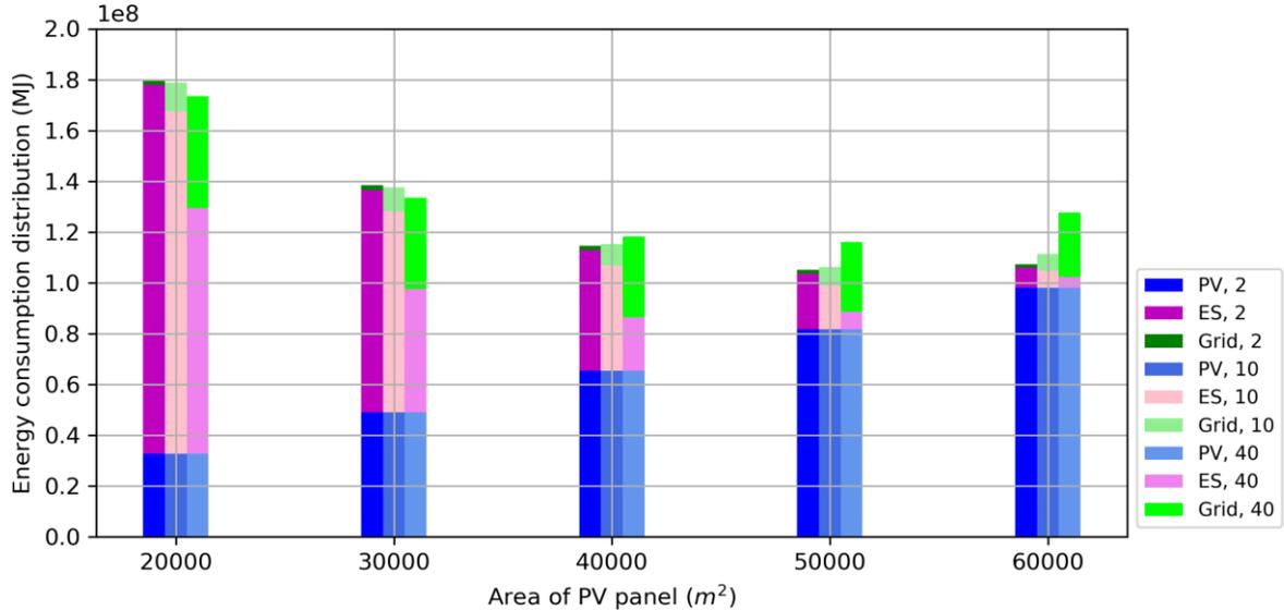
**Fig. 21.** Energy composition of PV panel, electricity storage and power grid.
