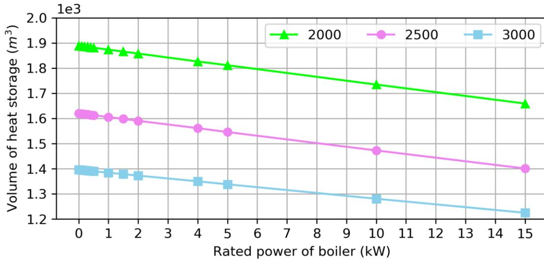
**Fig. 13.** Relationship between design capacity of heat storage and biomass boiler at different design areas of the solar thermal collector.
