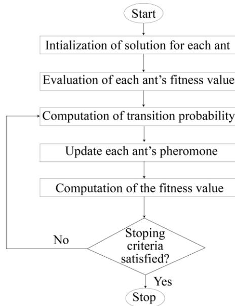
**Fig. 2.** Process flow of ACO.
