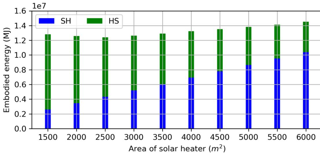
**Fig. 7.** Embodied energy distribution between solar thermal collector and heat storage.
