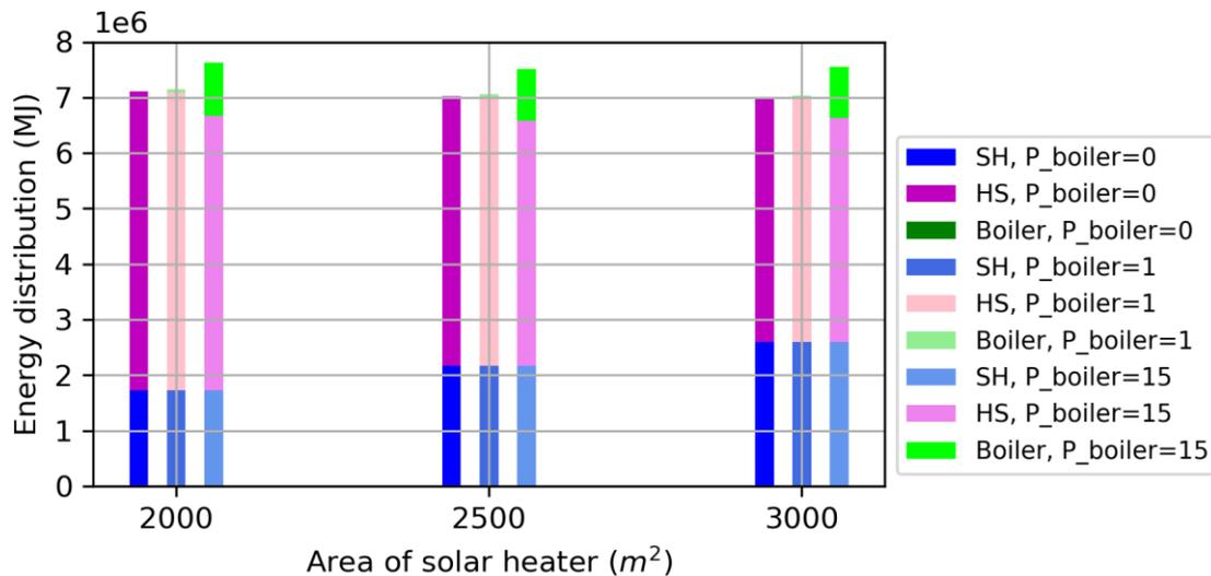
**Fig. 14.** Energy composition of solar thermal collector, heat storage and a biomass boiler.
