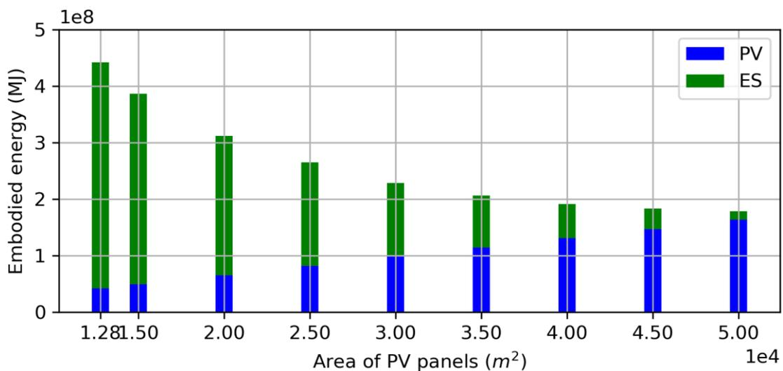
**Fig. 11.** Embodied energy distribution between PV panels and electricity storage.
