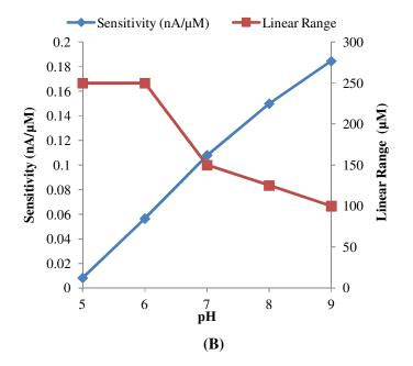
Fig. 4. A. Illustrates the effects of temperature upon the current response of the biosensor to injections of glutamate up to 275  $\mu$ M in 25  $\mu$ M steps. B. Illustrates the effects of pH upon the current response of the biosensor to the addition of glutamate. An applied potential +0.1 V vs. Ag/AgCl in 10 ml of 75 mM phosphate buffer solution containing 50 mM NaCl was used.
