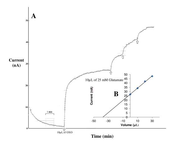
Fig. 5. A. Amperogram obtained using a GLDH-CHIT-MB-SPCE with a solution containing 10  $\mu$ L of a dissolved OXO cube; arrows indicate additions of 10  $\mu$ L of 25 mM glutamate into a 10 mL volume. Measurements taken 1.5 min after each addition. **B.** Typical standard addition calibration plot obtained with a solution containing a dissolved OXO cube using a GLDH-CHIT-MB-SPCE
