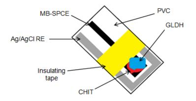
**Fig. 1.** Diagram of proposed biosensor strip; the insulating tape defines both the WE and RE. CHIT is then drop-coated and allowed to dry, followed by GLDH. All studies were conducted using a separate Pt wire counter electrode
