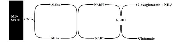
**Fig. 2.** Schematic displaying the interaction between the immobilized enzyme GLDH and glutamate at the surface of the electrode and the subsequent generation of the analytical response
