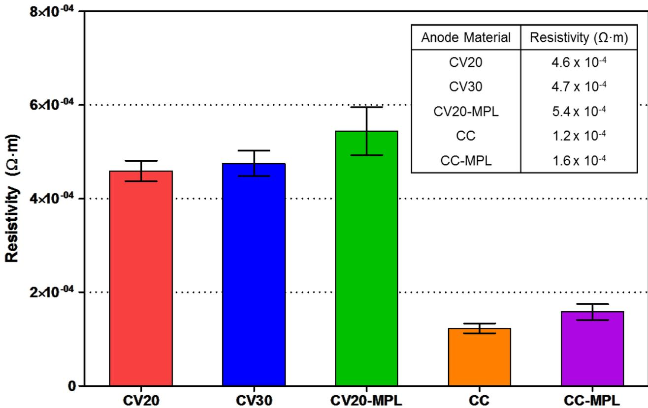
Figure 5. Electrical resistivity of each anode material
