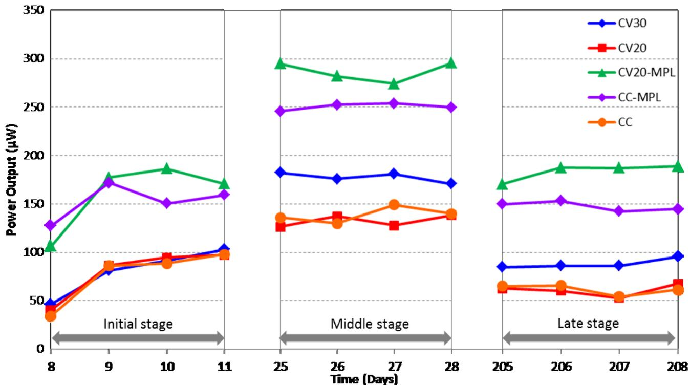
Figure 6. Power production from MFCs with different anode materials in different stages of the work; temporal profile
