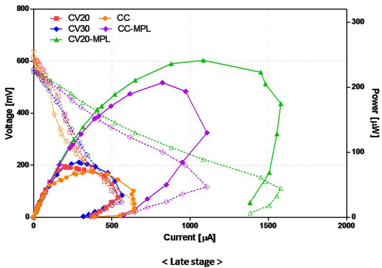
Figure 2. Power curves of different anode materials
