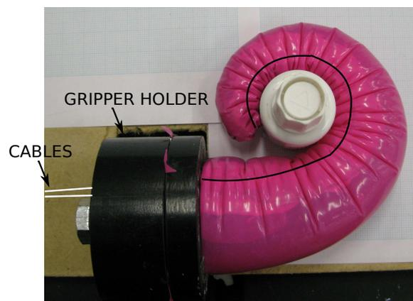
Figure 5.7: HS gripper in its stiff, bent state, when force is applied to its two cables (both are visible in white on the left of the picture, while one is shown in black along the HS gripper body. The other cable is in the exact same position but on the flip side).
