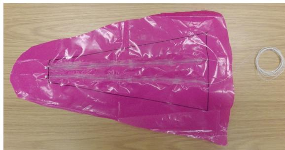
Figure 5.14: The silicone tubes have been glued to the corona treated polyethylene sheet, on which the edges of the cone have been stamped. The heat sealer is used to seal the edges together and then the cone is reversed inside out
