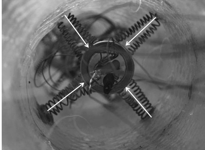
Figure 2.15: Cross-section view of the arrangement of transverse actuators in the SSSA artificial muscular hydrostat, the white arrows point towards the direction of movement of the SMAs: once they are given current, the SMAs coils contract and reduce the diameter of the cross-section. Figure from [Laschi et al., 2012], used with permission of Taylor & Francis.
