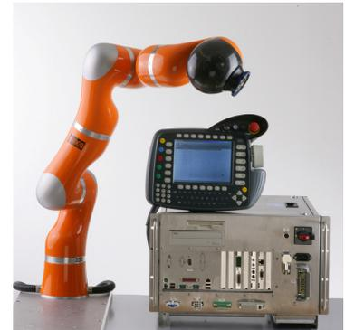
Figure 3.4: The LWRIII: its most salient features are the joint-integrated power and signal processing electronics including torque sensors mounted on the gear box output in all joints. Figure from [Bischoff et al., 2010], used with permission of Dr Bischoff.
