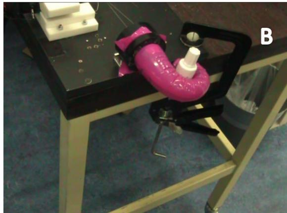
Figure 5.31: Grasping raspering without resting on table. A: the object is held by the human B: the gripper has successfully grasped the object. Figure from [Giannaccini et al., 2014], used with permission of Springer.
