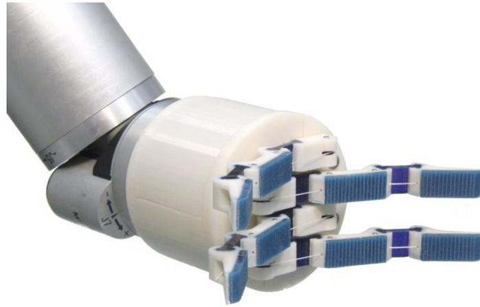
Figure 2.8: SDM hand. The hand is compliant in the workspace of the three link fingers. However, due to the inherent rigidity of the links and to their mechanical coupling between the finger links, the workspace of the SDM hand is inherently limited. Hence, the hand can adapt to external objects but retains movement constraints due to its mechanical structure. Figure from [Ma et al., 2013] ©2013 IEEE
