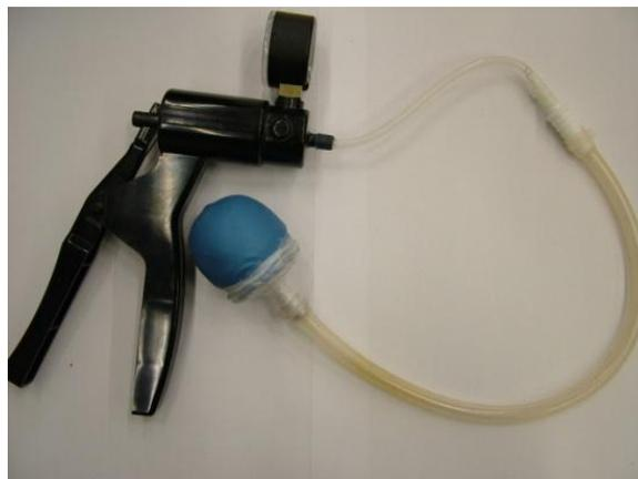
Figure 5.3: BRL reproduction of the University of Chicago universal robotic gripper built to test its functionality. This device is a good example of multidirectional compliance. Due to the lack of fixed shape in its flaccid state, there are no mechanical constraints which hinder its adaptation to an external object [Brown et al., 2010]
