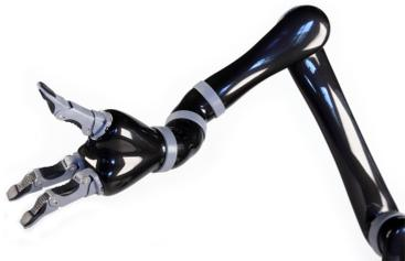
Figure 3.2: The Jaco arm is commercially available and used by disabled and elderly persons. Figure from [Maheu et al., 2011] ©2011 IEEE.
