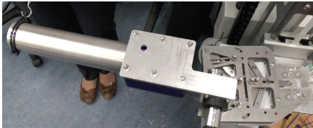
Figure 4.8: The INTRO-BRL robot arm link after a collision, when the HDF has been triggered and motor and link are decoupled. The flat metal plate and the blue box underneath it are the fixtures which hold together the HDF and the arm link
