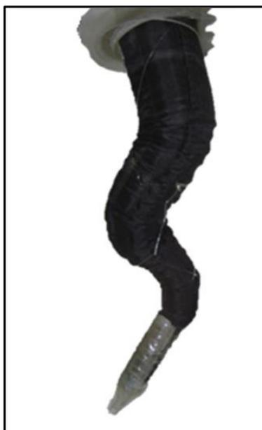
Figure 5.2: One of the possible configurations of the STIFF-FLOP manipulator. Figure from [Maghooa et al., 2015], ©2015 IEEE
