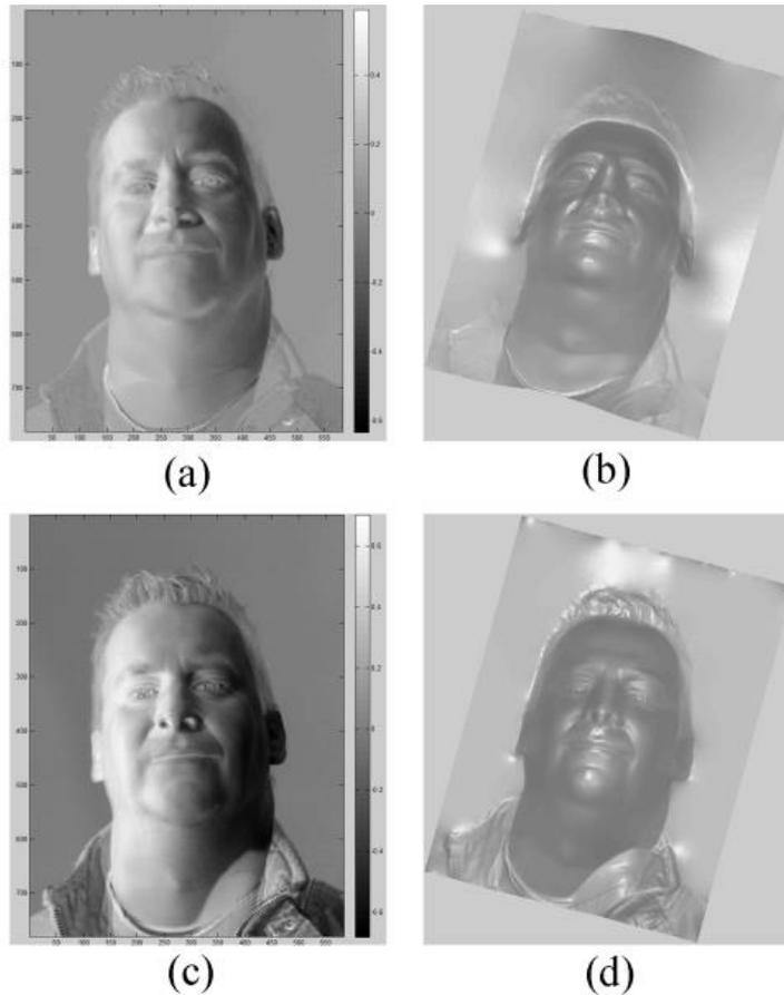
**Figure 6.13 A comparison of 3D face reconstruction between the two-source PS and standard four-source PS. (a) and (b) are the  $x$  gradient image and the depth image from the two-source PS while (c) and (d) are from the four-source PS.**
