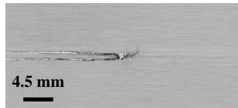
(a)  $[45/90/-45/0]_{4s}$ , Central double  $0^\circ$  ply, 14.2 kN (b)  $[45/90/-45/0]_{4s}$ , Single  $0^\circ$  ply, 14.2 kN
