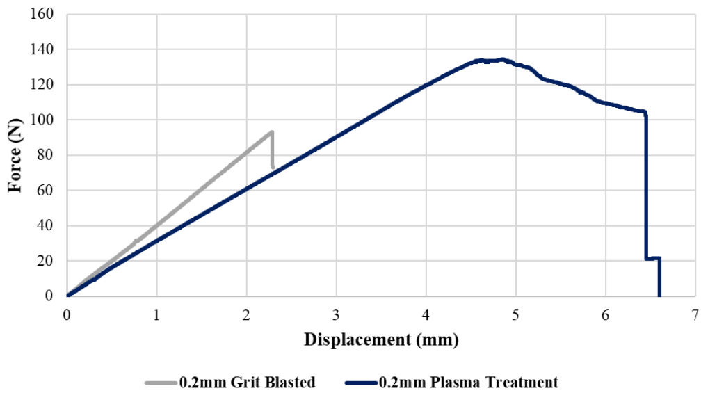
Figure 6 - Typical load displacement curves for the 0.2 mm nominal adhesive thickness DCB cases.
