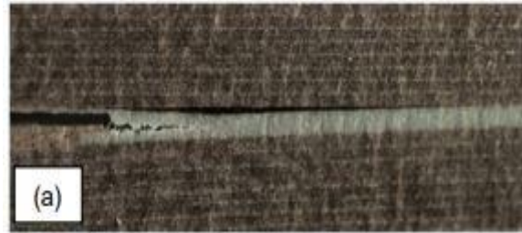
Figure 1 - Example of double delamination [9].
