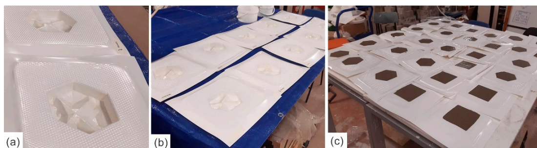
Figure 3. Photographs illustrating the casting process. (a) Vacuum formed mold from negative CNC'ed model (b) Vacuum form molds (c) Concrete casting.
