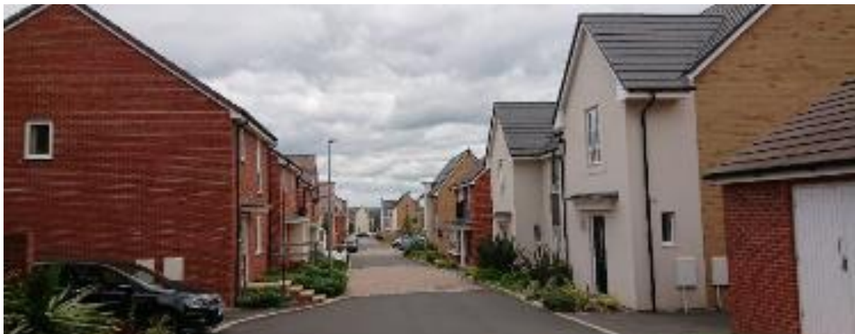
Image CH12: A tertiary street in Phase 3 with narrowed shared space carriageway access, predominantly brick finish, open front gardens and side (rather than frontage) parking. This creates an intimate street character.
