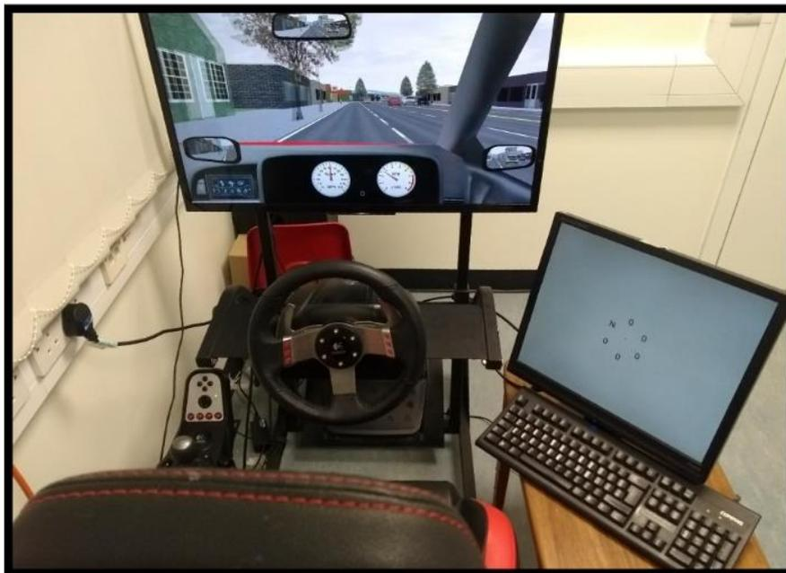
Figure 4.1. Experimental set up. Participants partook in simulated driving following a high load search task or a low load search task presented on a monitor, or a passive viewing task, where participants watched the roadway ahead.
