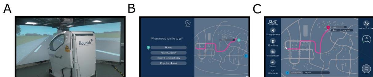
*Figure 6.2.* The driving simulator and human-machine interface (HMI). **(A)** The exterior of the Lutz Pod in front of three large forward projector screens. **(B)** The HMI screen during journey set up. **(C)** The HMI default screen during the journeys.
