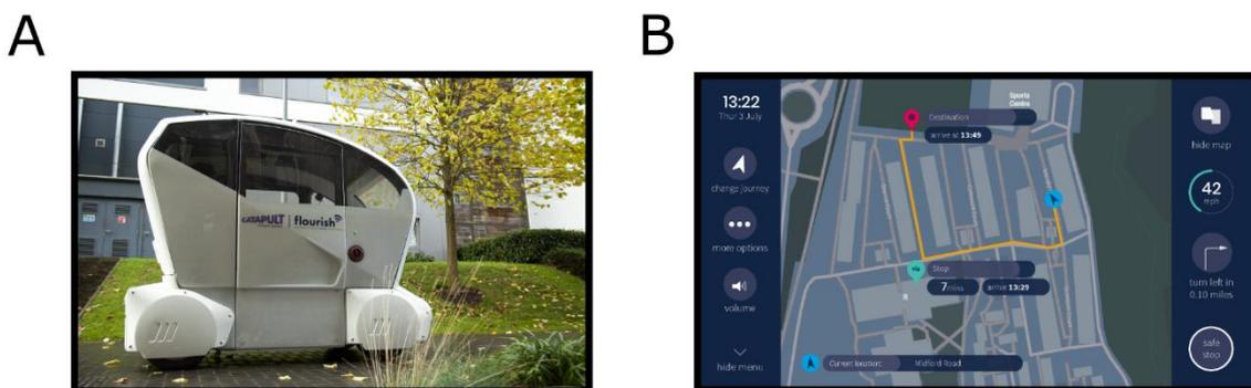
Figure 5.1. Autonomous vehicle and human-machine interface. **(A)** Autonomous Pod utilised during the study. **(B)** Human-machine interface display during the journey.
