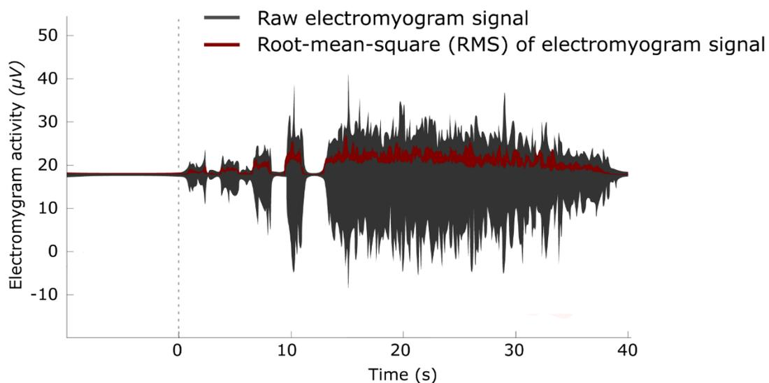
*Figure 1.3.* Electromyogram (EMG) signal. An example graph depicting the root-mean-square (RMS) envelope (red) overlaying the raw EMG signal (black). Dashed line represents stimulus onset.
