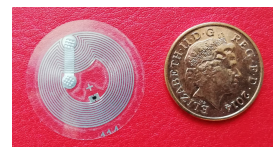
Figure 6: NFC sticker size compared to a penny
