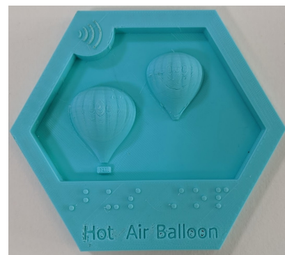
Figure 7: 3D printed textured tile with embedded NFC tag
