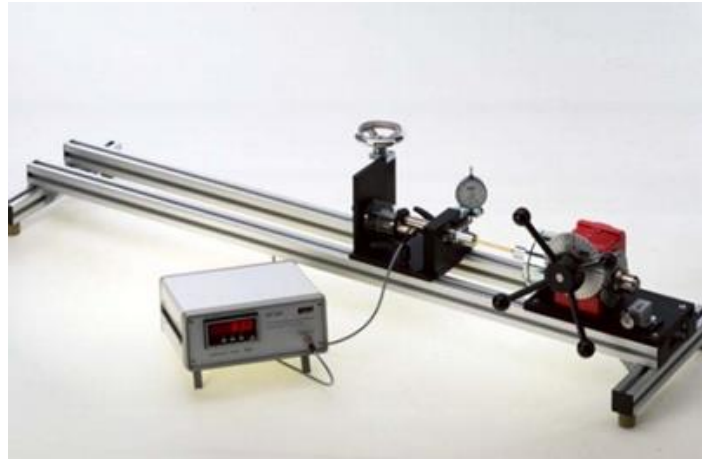
Figure 33. Gunt WP500 torsional tester at University of the West Indies.
