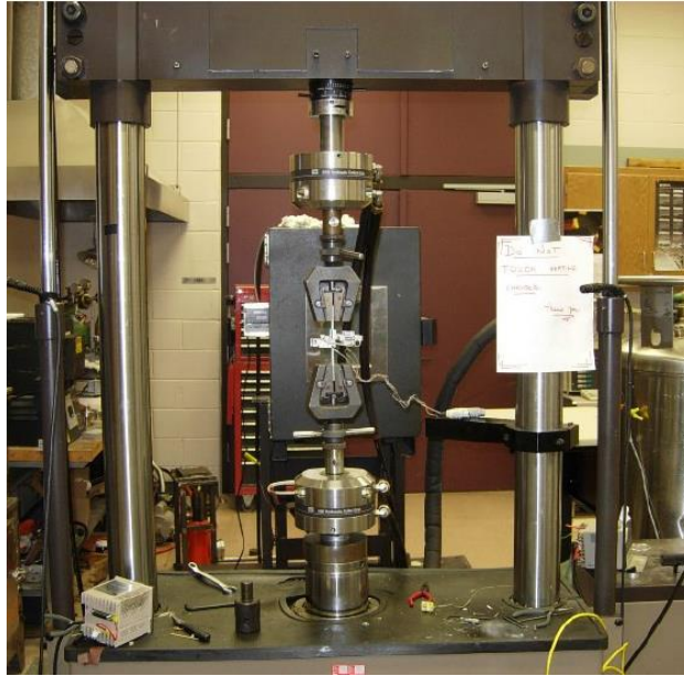
Figure 31. Tensiometer with ASTM D638 type-V dog-bone Sample. University of the West Indies, Tested on 6/10/2016.
