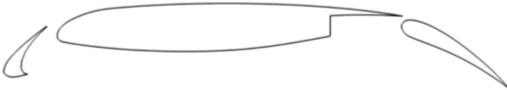
**Figure C.1.** MD 30P30N three-element model geometry. (Khorrami et al., 2004; Murayama et al., 2014; Choudhari and Lockard, 2015)
