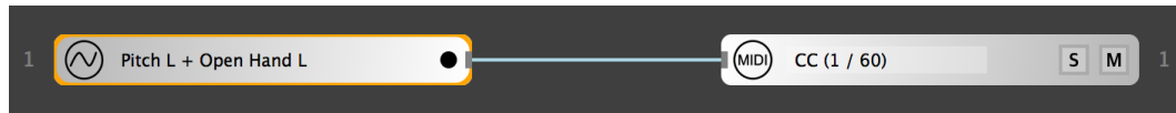
Figure 5.5.: Left hand pitch (movement) and Open Hand posture (qualifier) control the value of a MIDI CC message.
