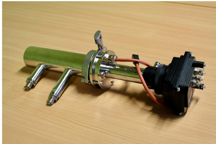
(c) Pegasor M-sensor particle mass and particle number sensor.
