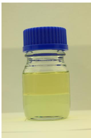
**Figure 4.2:** Qualitative check for blend stability for E20 fuel blend [41].
