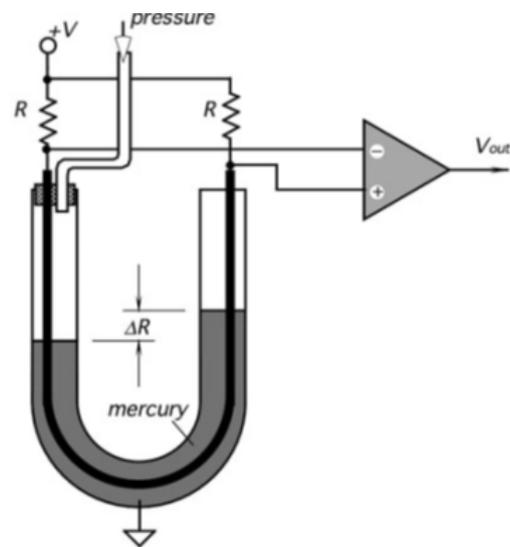
Figure 3.4: Shows the design of a mercury pressure sensor [84].
