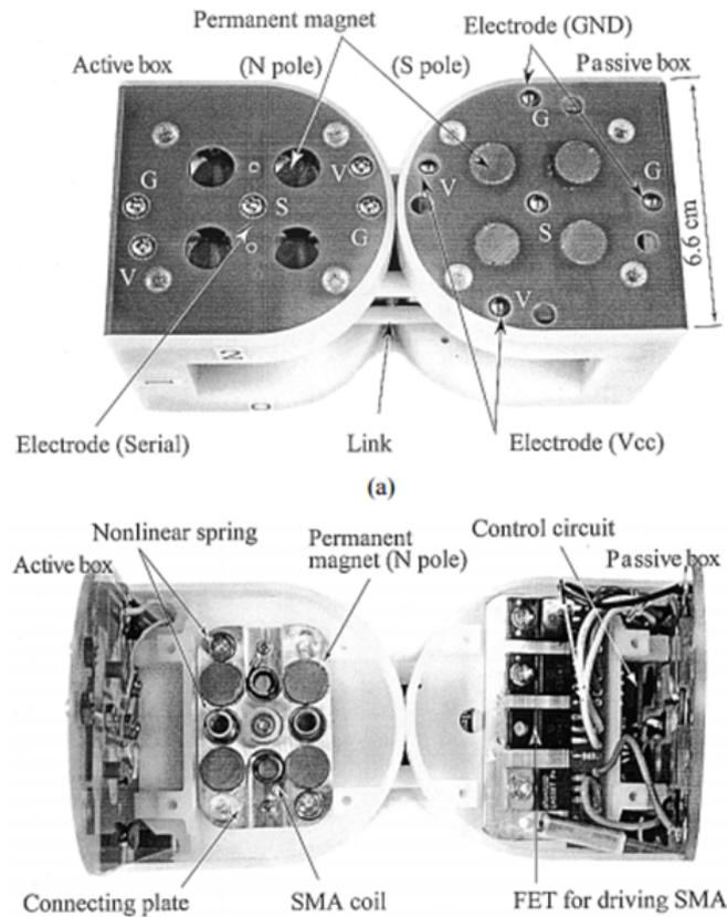
Figure 2.10: Shows the individual module that is the constituent of M-Tran [177].
