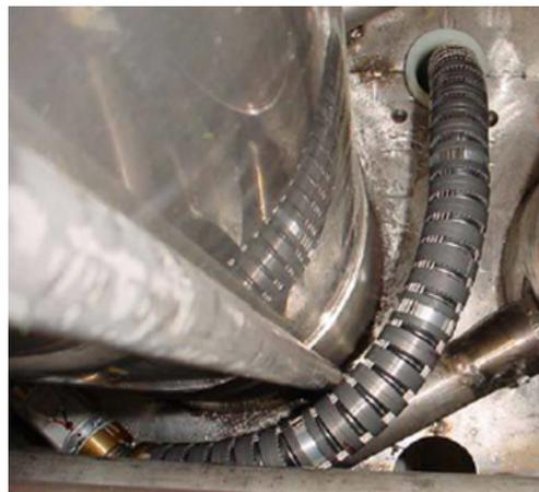
Figure 2.4: Shows a snake arm robot repairing a pipe at the Ringhals nuclear power plant [33].
