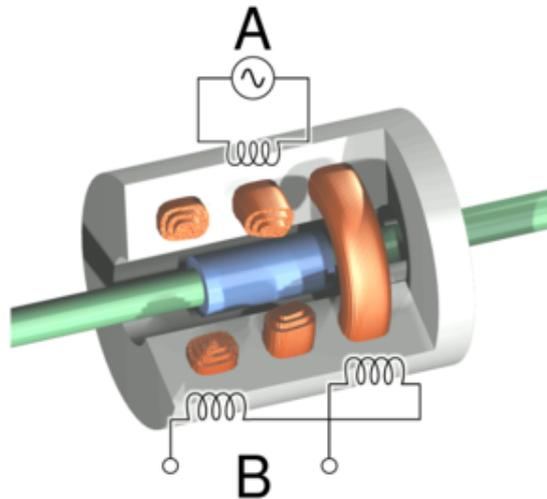
Figure 3.1: Shows the design of an LVDT sensor [252].
