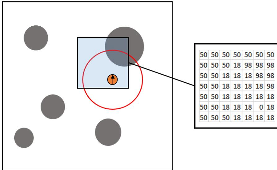
Figure 5.1: Shows a robot navigating an obstacle filled environment with an example occupancy grid.
