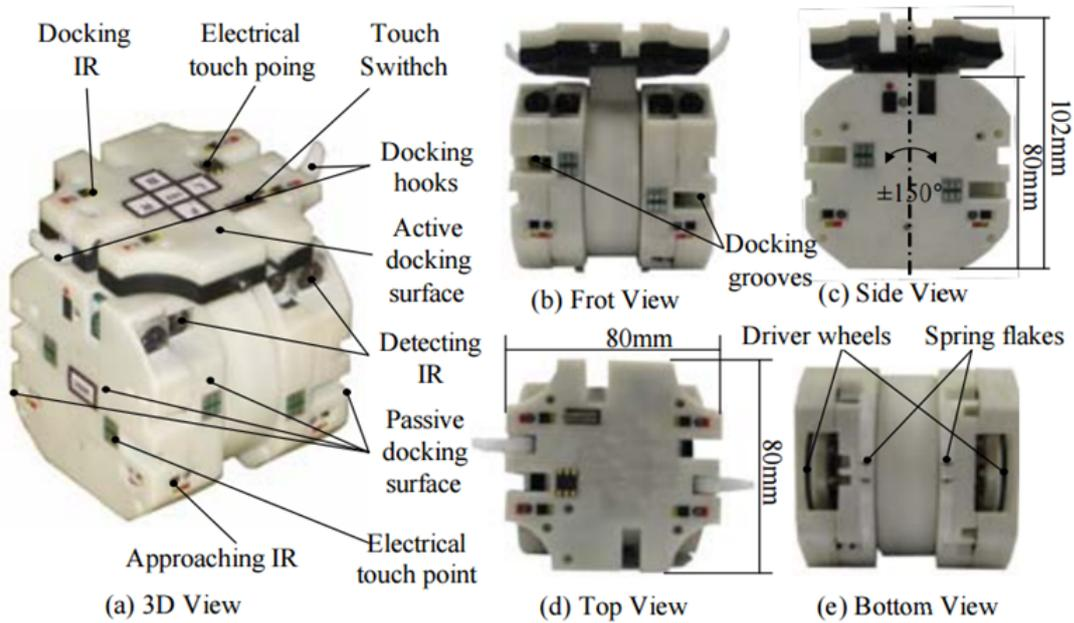
Figure 2.11: Shows the individual modules that comprise Sambot [245].
