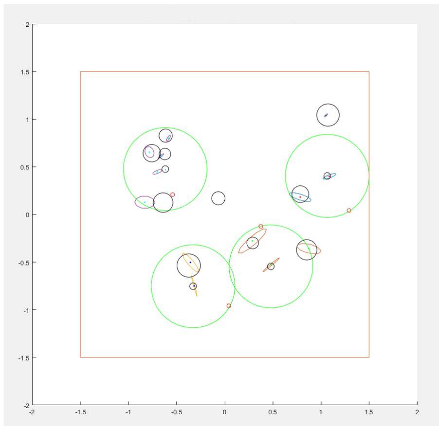
Figure 6.1: The SLAM map generated by the robots. The ellipses and dots near obstacles represent the error ellipse and estimated position of the landmarks. Ellipses around robots represent their uncertainty in their own position. Circles around robots represent their sensor range.
