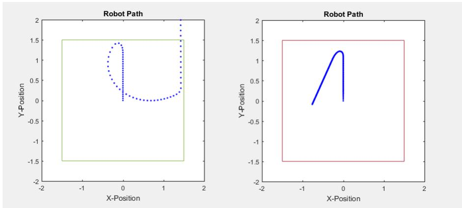
Figure 5.3: Illustrates an undesirable path (left), due to the looping back on itself and leaving the arena, and a desirable path (right).
