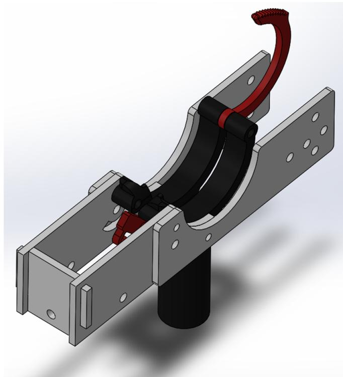
Figure 4.11: Shows a three dimensional rendering of the grapple's design. The red components show the locking mechanism, comprising of the ratcheted swivel and lock pin. In black the main body of the grapple is shown. Finally in white, the support (left) and balance (right) side and back pieces are shown.
