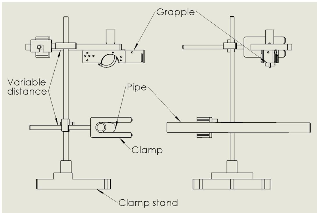
Figure 4.13: Shows the two dimensional layout of the test rig used for the consistency verification.
