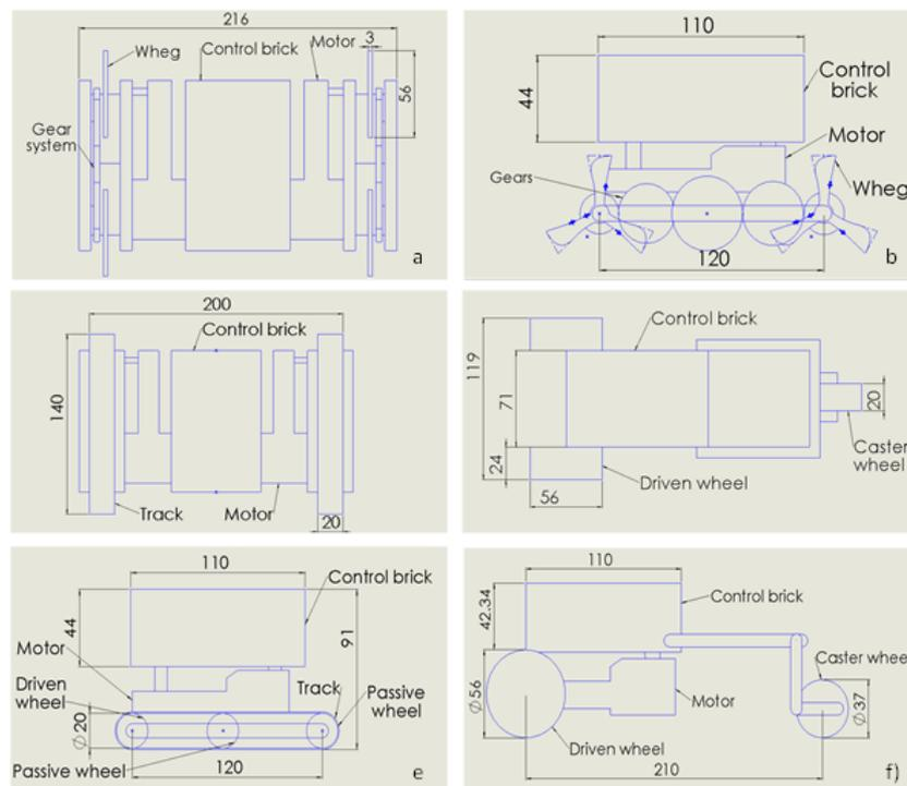
Figure 4.7: Shows the layout of each robot used; all units are in mm. The front of the robot is on the left for side views and upwards for birds eye view diagrams. a) & b) show the top and side views of the whegged robot respectively. c) & e) show the side and top view of the tracked robot respectively. d) & f) show the side and top view of the wheeled/ spherical robot respectively.
