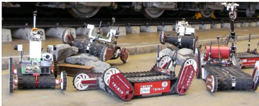
Figure 2.6: Shows the quince robots used for search and rescue in Japan [178].
