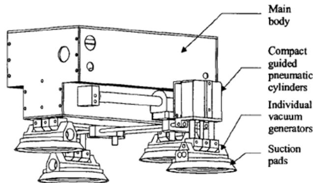
Figure 2.1: Shows the design of the Robicen III [210].
