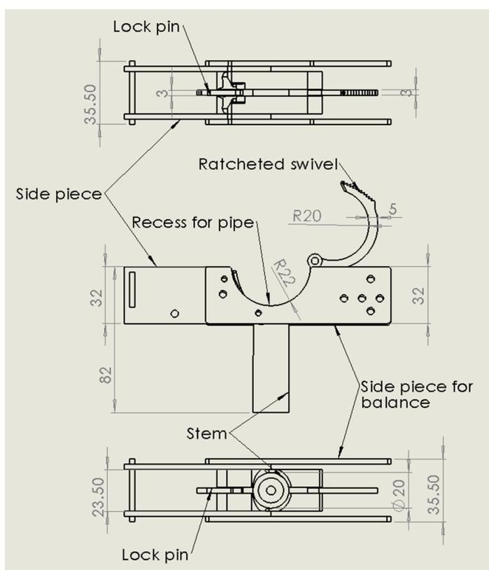
Figure 4.10: Shows the design and dimensions of the grapple in two dimensions.
