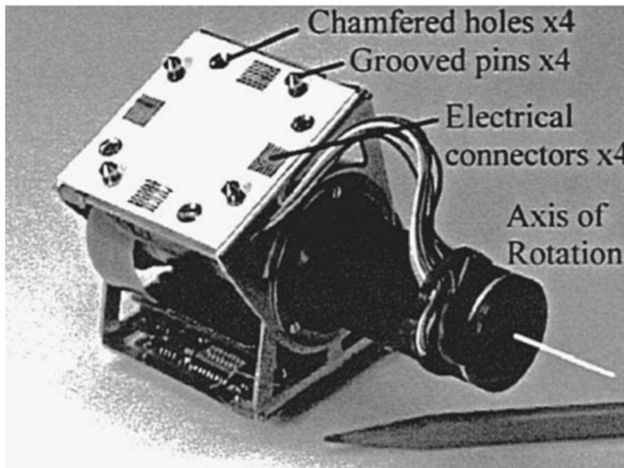
Figure 2.12: Shows the individual modules of the Polybot robot [266].
