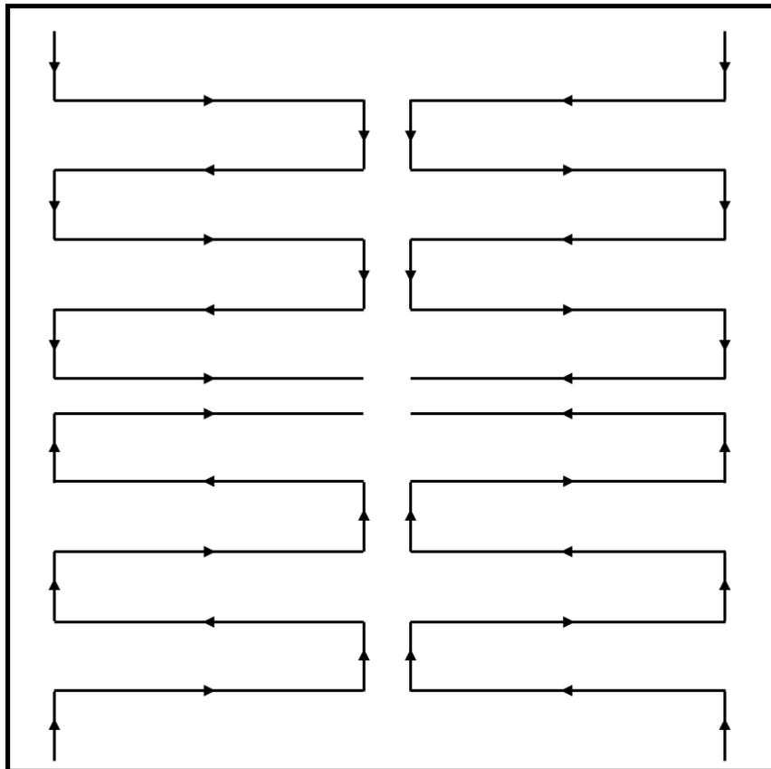
Figure 6.4: An example of a potential implementation of a perfect raster for four robots.
