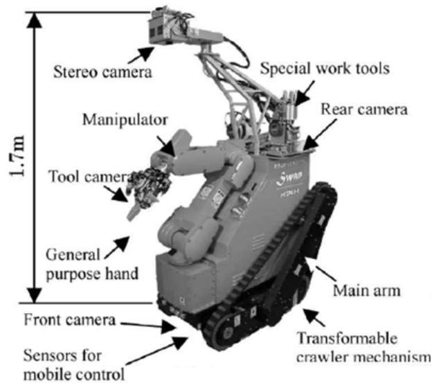
Figure 2.7: Shows the SWAN robot used for nuclear disaster prevention [105].
