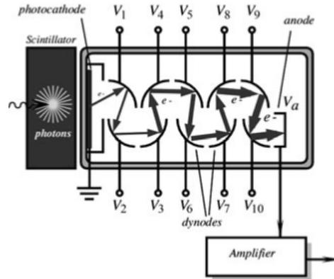
Figure 3.2: Shows a the design of a scintillator detector, with a photo multiplier [84].
