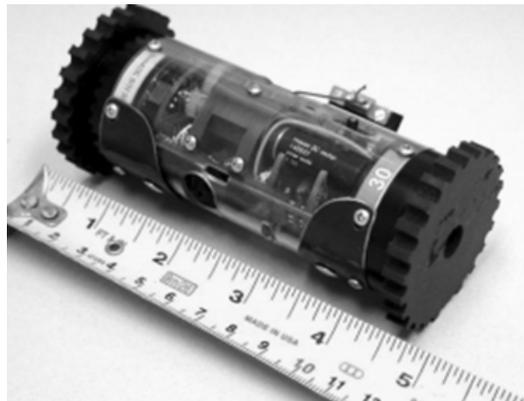
Figure 4.6: Shows the scout robot, a small robot capable of jumping 35cm into the air using a bent spring [229].
