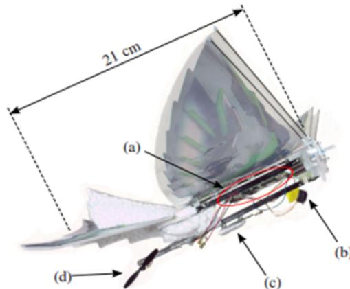
Figure 4.4: Shows the 13 gram ornithopter with (a) Control electronics, (b) a visual sensor, (c) a battery, and (d) a propeller [10].
