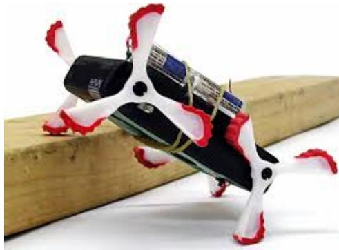
Figure 4.1: Shows a small whegged robot, capable of surmounting obstacles greater than the wheg diameter [137].
