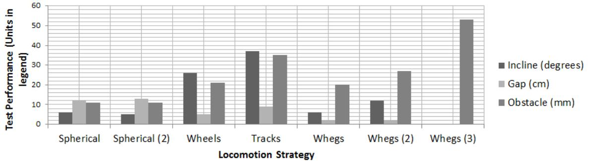
Figure 4.8: Shows the results from the comparative test. The (2) denotes addition traction tested on spherical and whegged robots. The (3) denotes an additional obstacle clearance test carried out with whegged robot with increased traction; in this test only the front whegs were required to surmount the obstacles.
