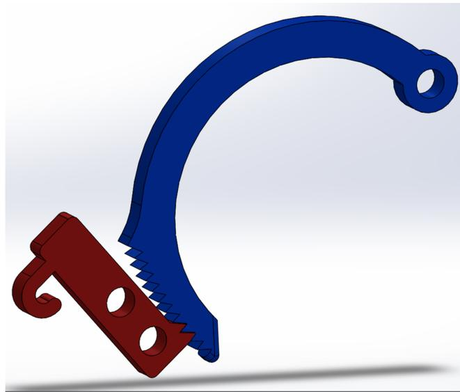
Figure 4.9: Shows the design of the ratcheted swivel (right) and the lock pin (left) that are used to secure the grapple to pipe work.
