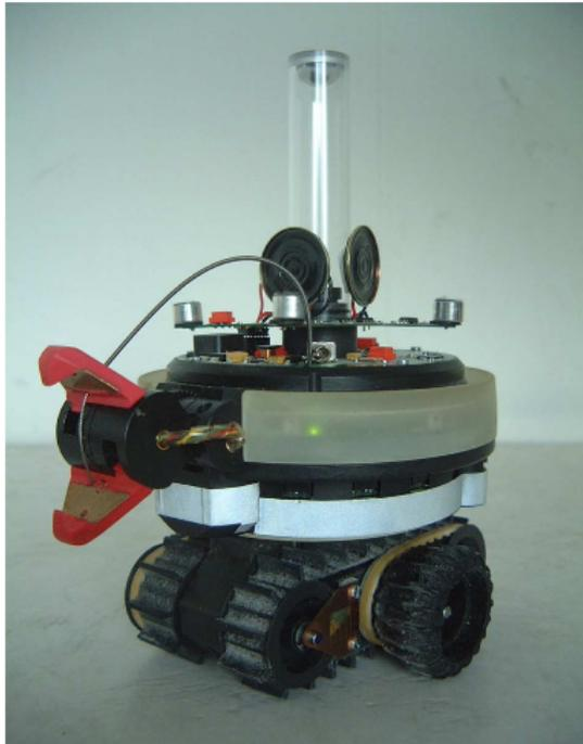
Figure 2.8: The swarm-bot robot, used for homogeneous experimentation [67].
