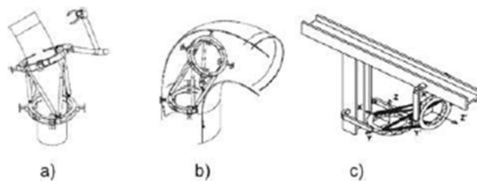
Figure 2.2: a) Shows the robot mode used to climb the outside of a pipe. b) Shows the mode used to climb through the inside of a pipe. c) Shows the additional of legs to enable the climbing of girders. [207]
