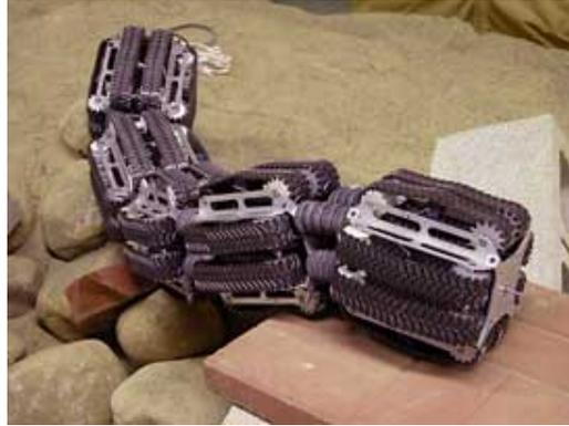
Figure 4.3: Shows the OmniTread robot utilising its serpentine design to overcome debris [6].
