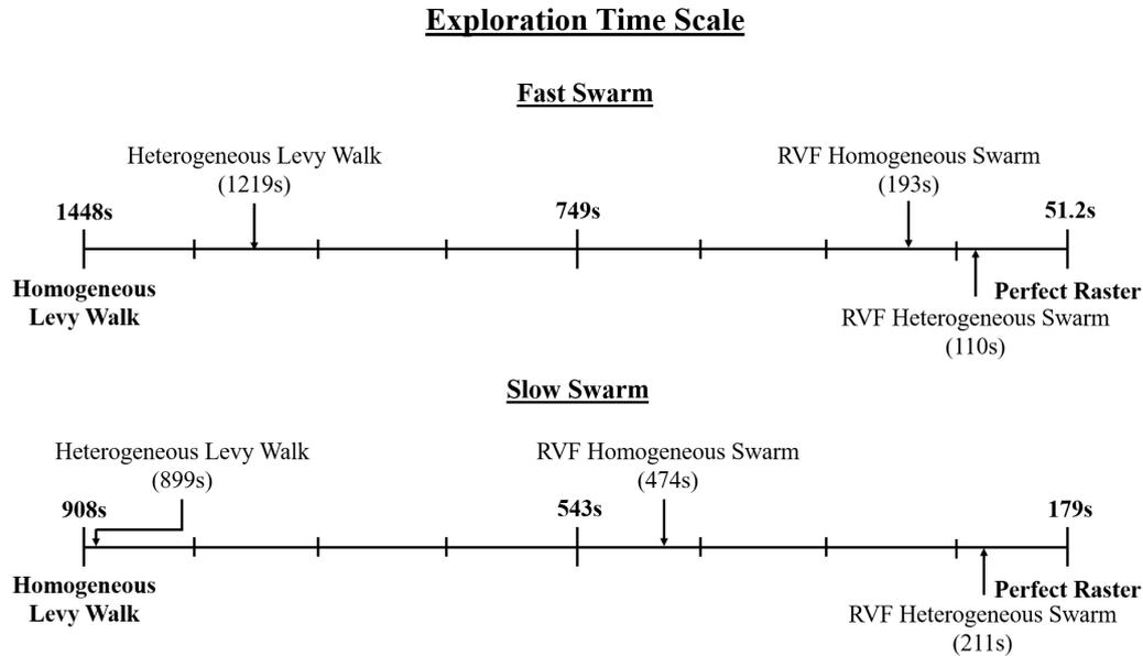
Figure 6.7: Shows where exploration time of the RVF framework sits on the comparative scale.
