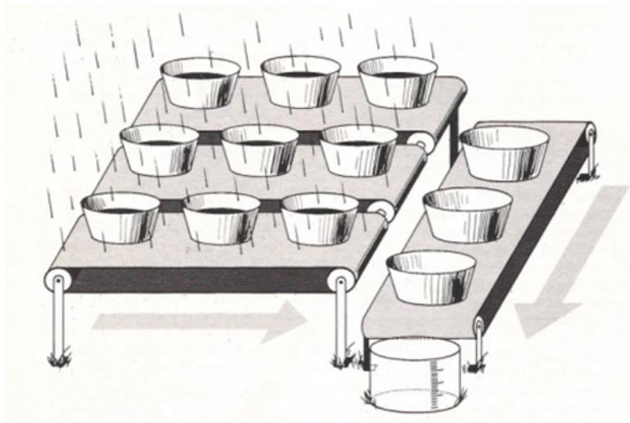
Figure 3.5: Shows how a CCD device operates with a simple analogy, where the water collected represents incident light and the buckets represent pixels [116].
