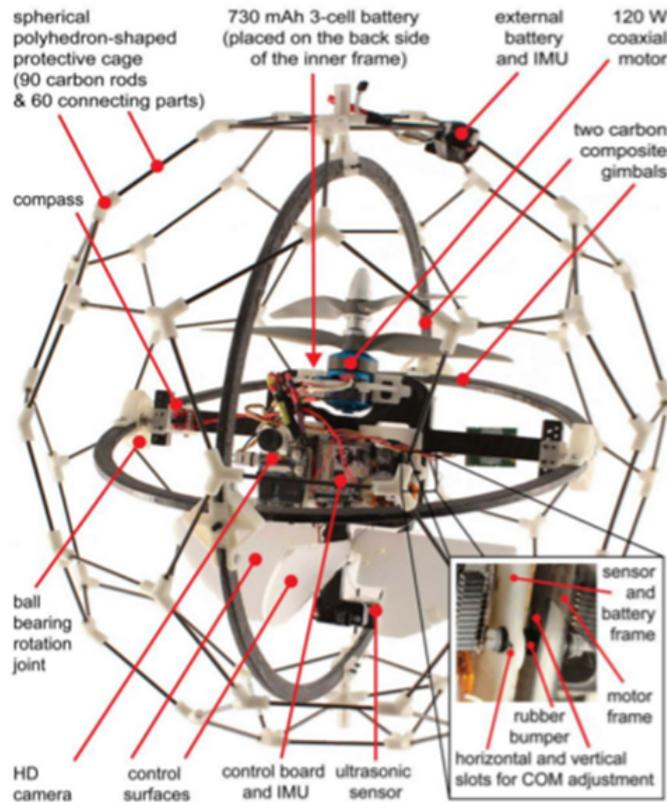
Figure 4.5: Shows the GimBall, a rotor craft able to fly through complex environments and survive multiple collisions [29].
