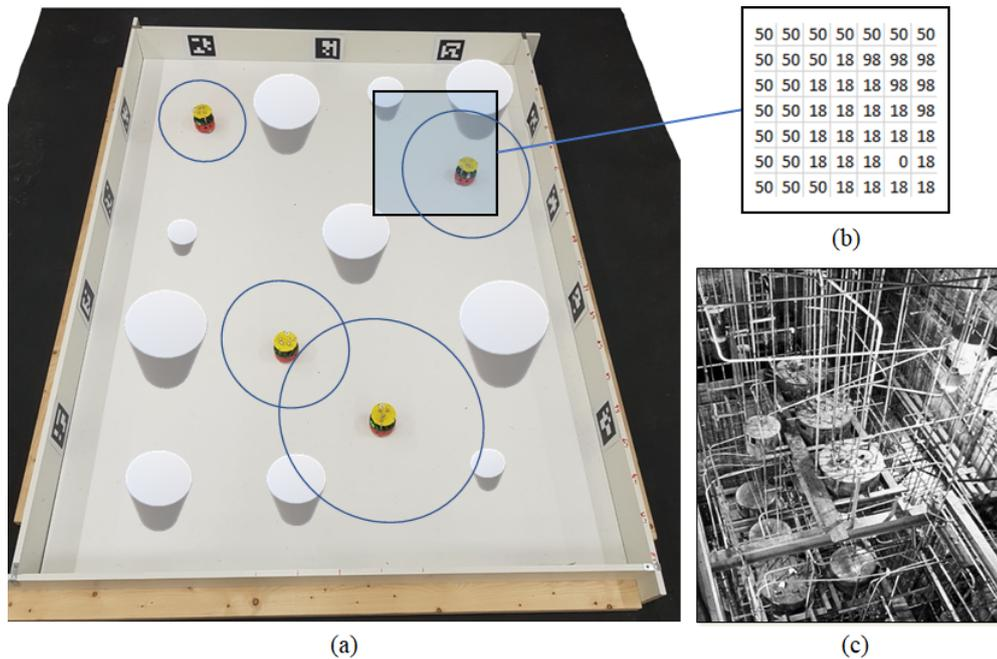
Figure 5.5: a) The arena in which the experiments were conducted, the virtual obstacles have been overlaid onto the environment. Sensor ranges are represented by rings around each e-puck. b) An example occupancy grid, after multiple updates. c) A photograph of a nuclear cave environment, taken before the cave was sealed.
