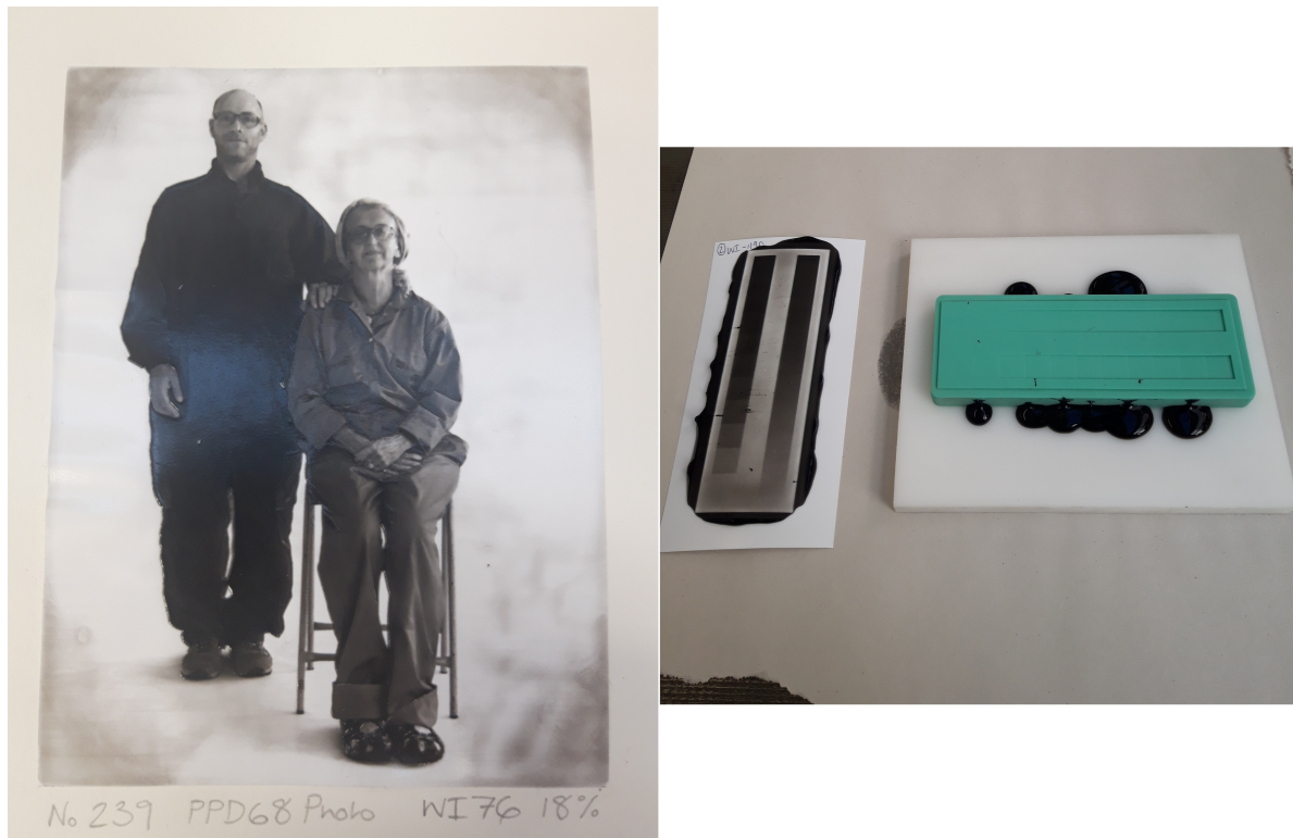
Figure 1. Left: Example of the Woodburytype printing process, mounted on card. The ink used has a pigment content of 0.015%. Right: Print next to the step-wedge printing plate, after being pulled. The ink used here has a pigment content of 0.025%.
