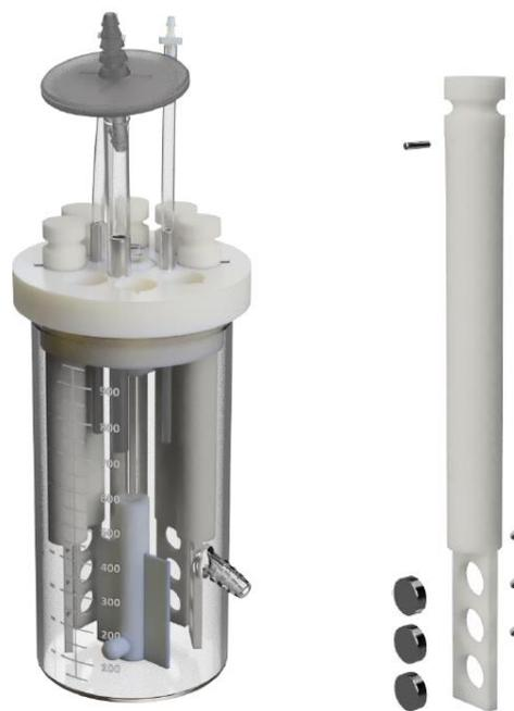
Figure 2.6: Assembled CBR reactor chamber (left) and a single coupon-holding rod (left) with coupons and securing screws (reproduced from BioSurface Technologies Corp, 2016)
