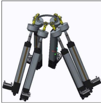
Fig. 9: "Classical 6-6 Gough-Stewart architecture with base diameter of 800 mm and platform diameter of 240 mm" [22]
