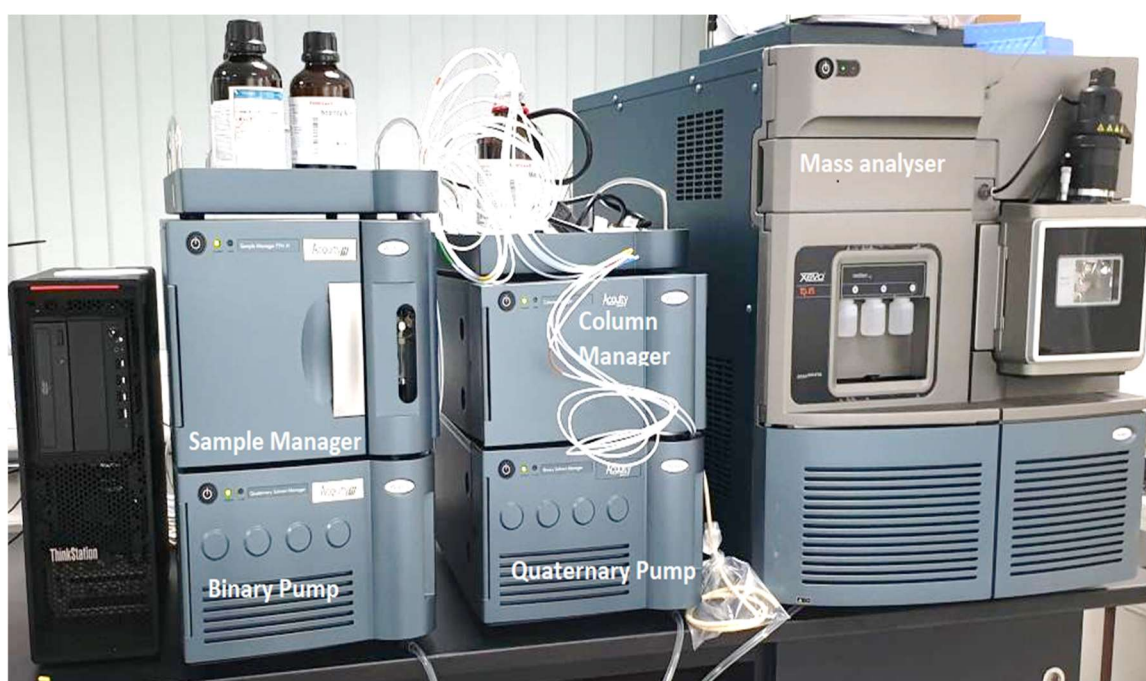
Figure 2. 1 The Waters Xevo TQSX Tandem Quadrupole Mass Analyser The components are a sample manager, Binary pump, an Acquity UPLC column manager, quaternary pump, and a mass analyser.
