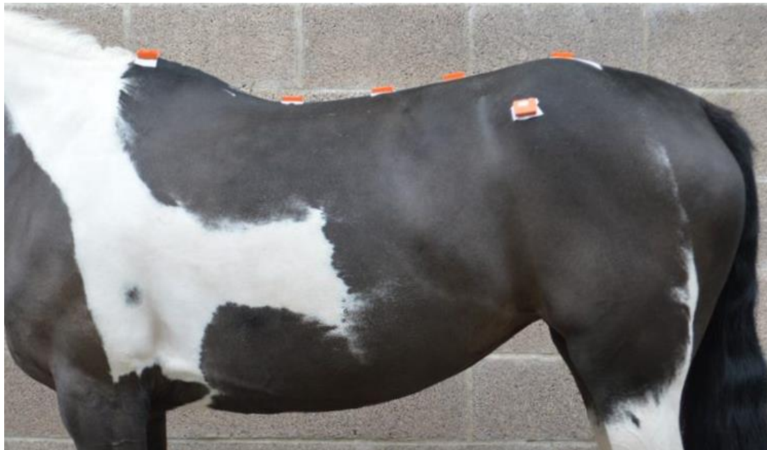
Figure 5.1 | The placement of the skin-mounted IMUs on the anatomical landmarks of the spinous processes T5, T13, T18, L3, and TS, and the LTC and RTC.
