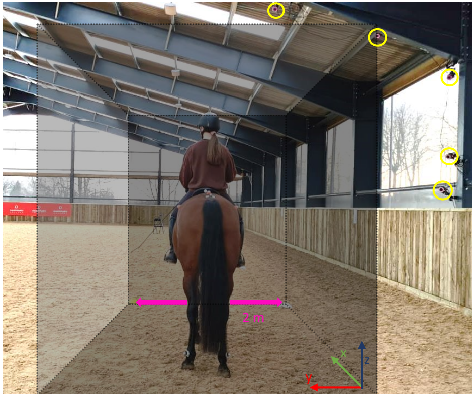
Figure 5.3 | The volume (2x6 m) to be captured by the optical motion cameras (encircled in yellow). The coordinate system was located on the right side of the volume.
