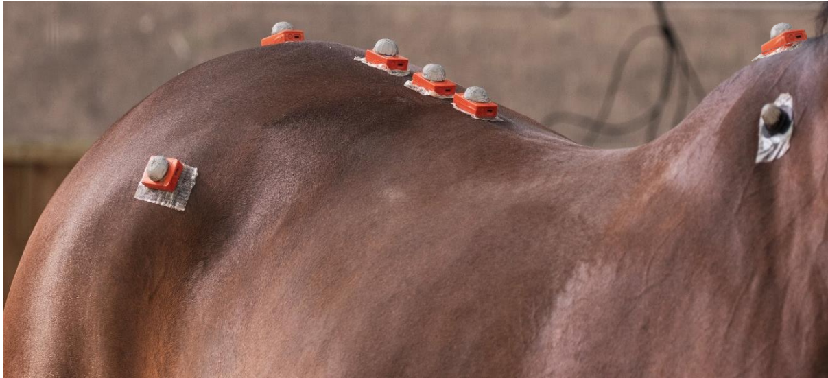
Figure 5.2 | The placement of the skin-mounted IMUs, with hemispherical markers on top, placed on the anatomical landmarks at T6, L1, L3, L5, and S3 and the LTC and RTC.
