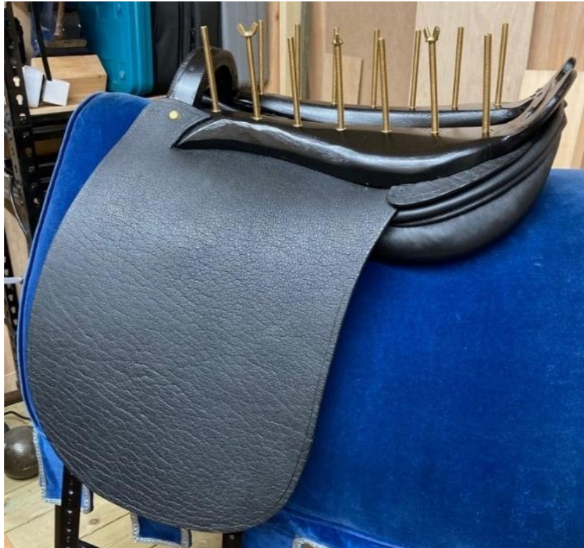
Figure 4.1 | The final design of the experimental saddle. The saddle was designed without a seat to allow optical motion capture of the midline of the horse's mid-caudal thoracic region. Metal pins were screwed into the saddle tree to allow additional weights to be attached to it.
