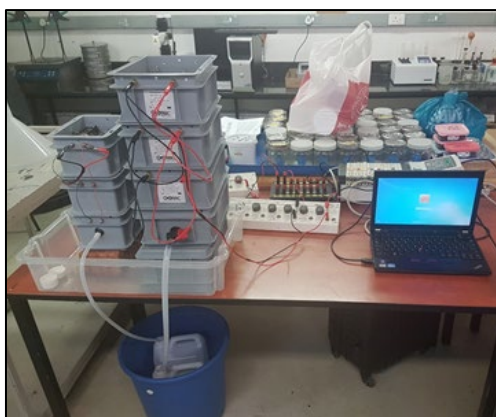
Figure 4.6: Lab facilities in the WASH Centre of UKZN, showing two cascades of the PEEPOWER system used for testing and training. Photo credit: UKZN WASH Centre.
