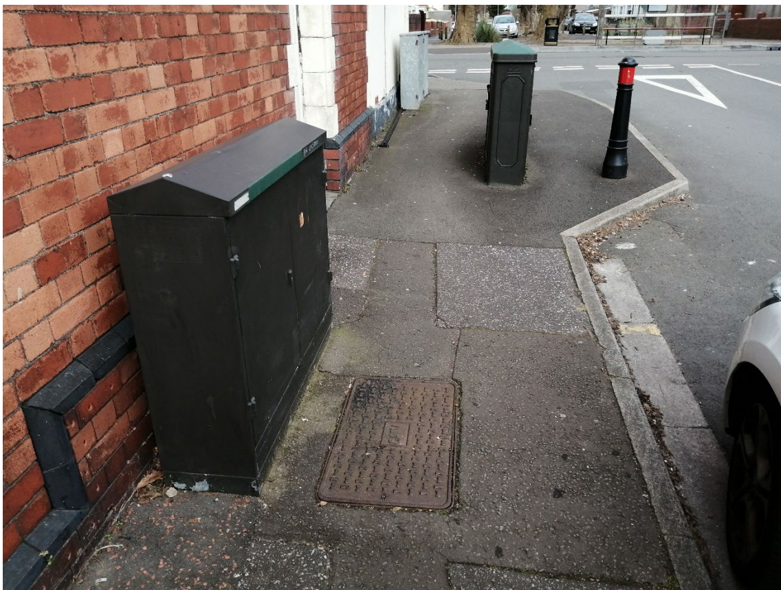
Figure 41: Chamberlain Street, illustrative example of 'street clutter' including utilities and bollard that restrict the effective clear width of the pavement
