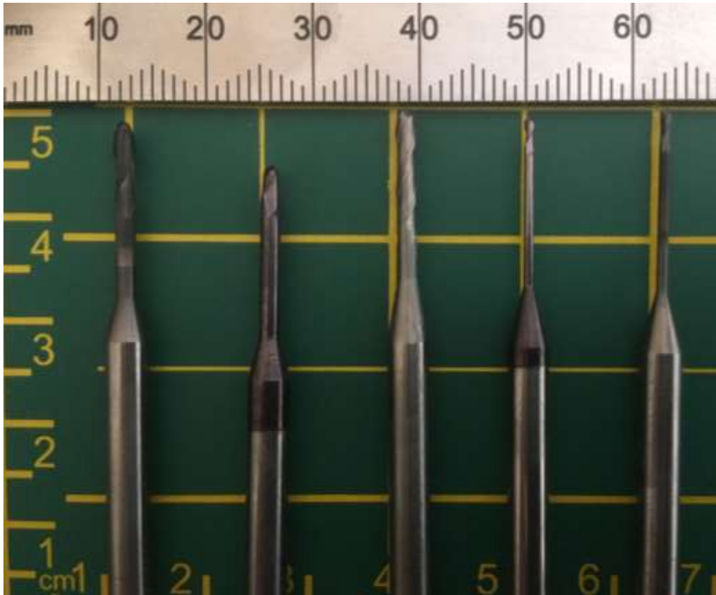
Figure 2-2: Typical Ball Nose End Mills Used in Machining Dental Restoration
