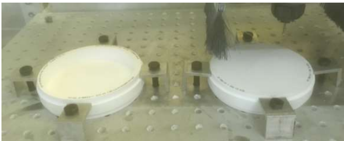
Figure 11: Pre-sintered zirconia disc inside the CNC router
