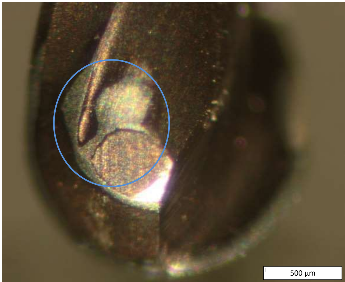
Figure 4-2: Example of Wear Occurring on Secondary Relief of Tool After Machining Pre-Sintered Zirconia
