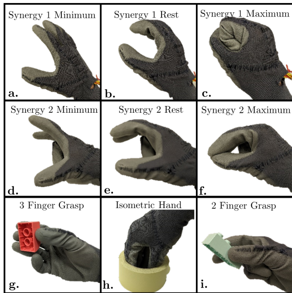
Fig. 3. Table depicting the various hand poses seen within the experiment with synergies 1 & 2 the desired movements for the idealised experiment
