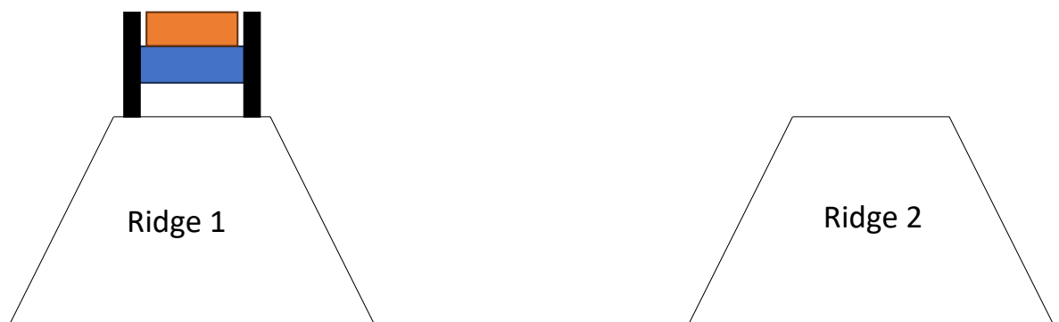
Figure 5-39 Showing how the Real-World Data was Collected (GSSI Antenna Direction of Travel is into the Page).
