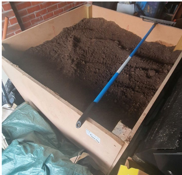
Figure 4-6 Showing the Final Rig with Topsoil in (Before Levelling)
