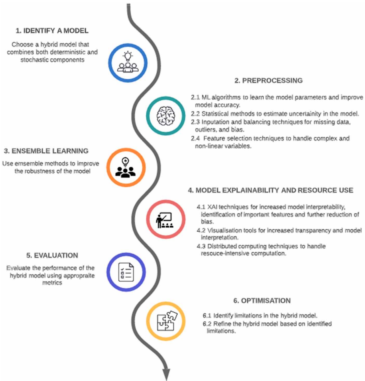
Figure 8 | A suggested workflow for deploying an explainable hybrid model that can effectively predict solids deposition in a gully pot.
