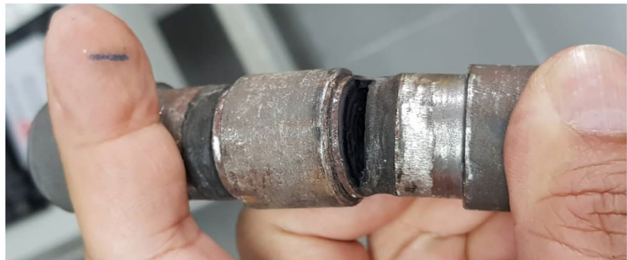
(c) Deformed and teared rubber specimen
