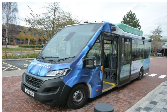
Figure 3: Phase One and Two electric, autonomous Mellor Orion minibus
