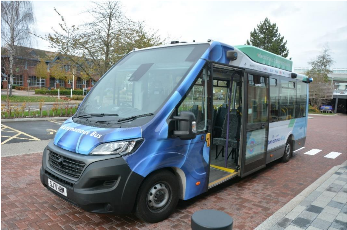
Figure 1: The electric autonomous Mellor Orion minibus used on Services 001 and 002
