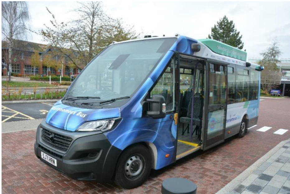
Figure 1: Electric, autonomous minibus used on Services 001 and 002
