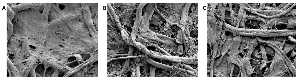
Fig. 4.3. Scanning electron micrographs of chromatography papers (x 500, 2.00 kV) A) Whatman No. 1, B) Whatman SG81, C) Whatman 3MM.
