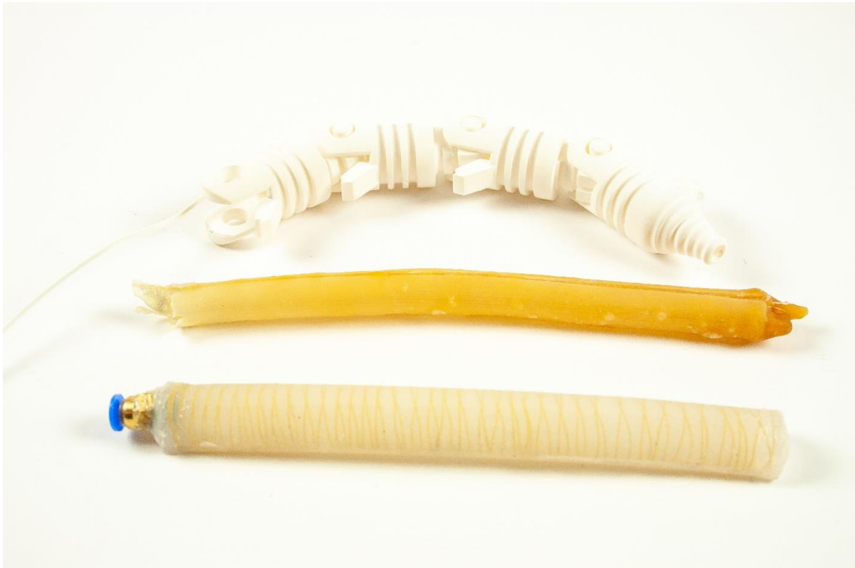
Figure 14 two different approaches: top - tendon, bottom - soft air
