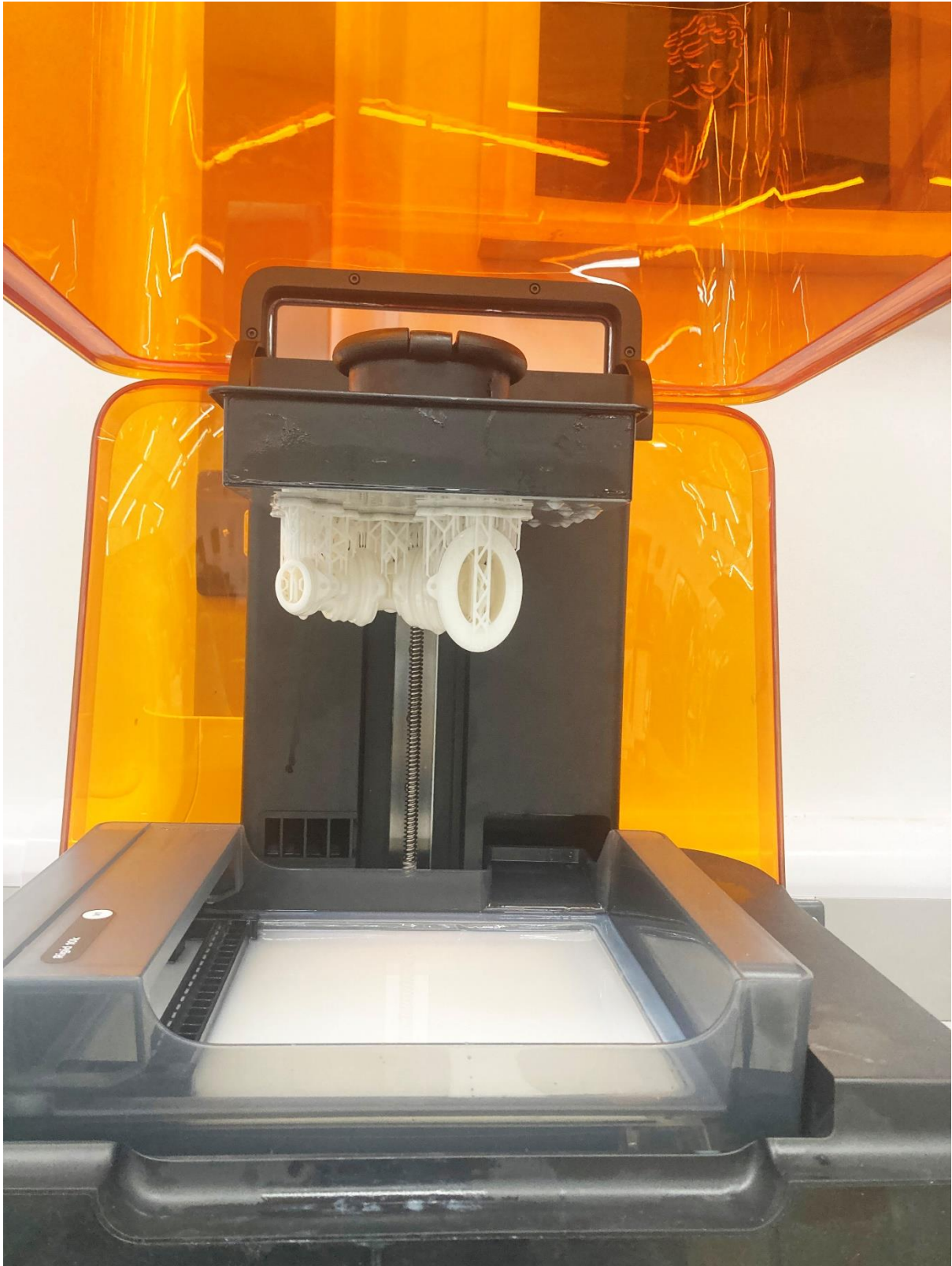
Figure 24 the trunk being printend in one piece, with the working hinges
