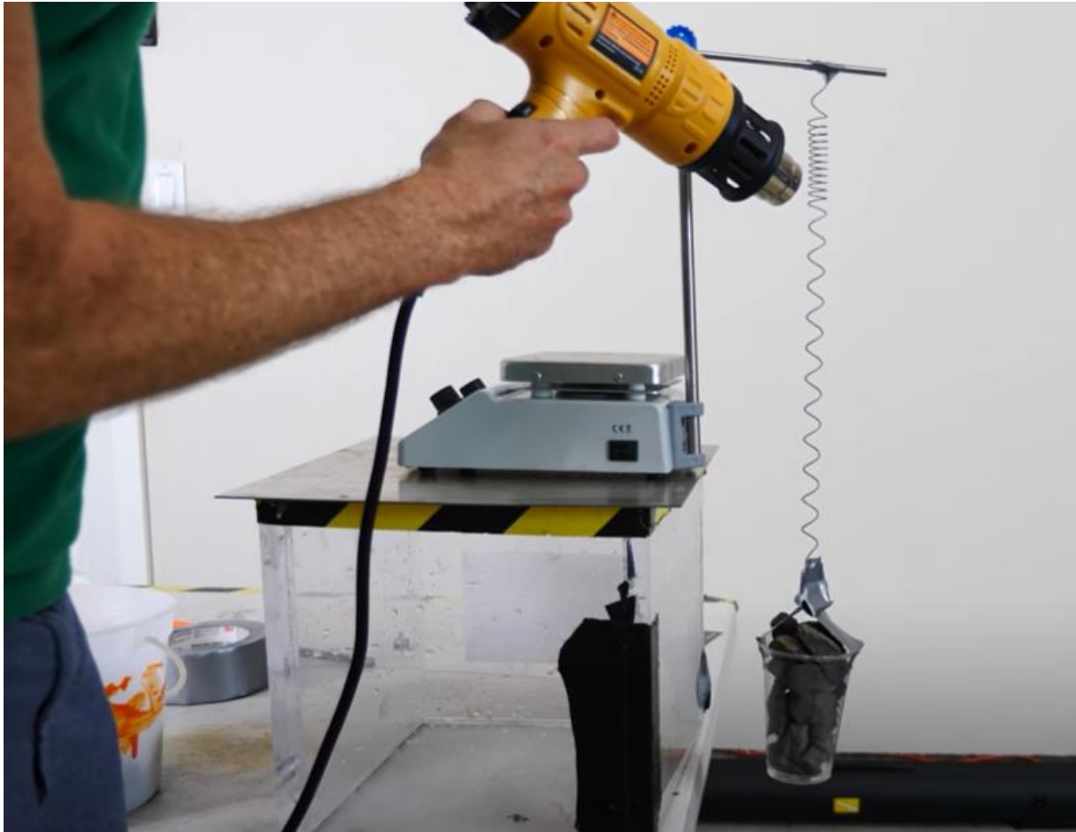
Figure 10 a Nitinol spring, source: https://www.youtube.com/watch?v=65r6Ztxi0EQ
