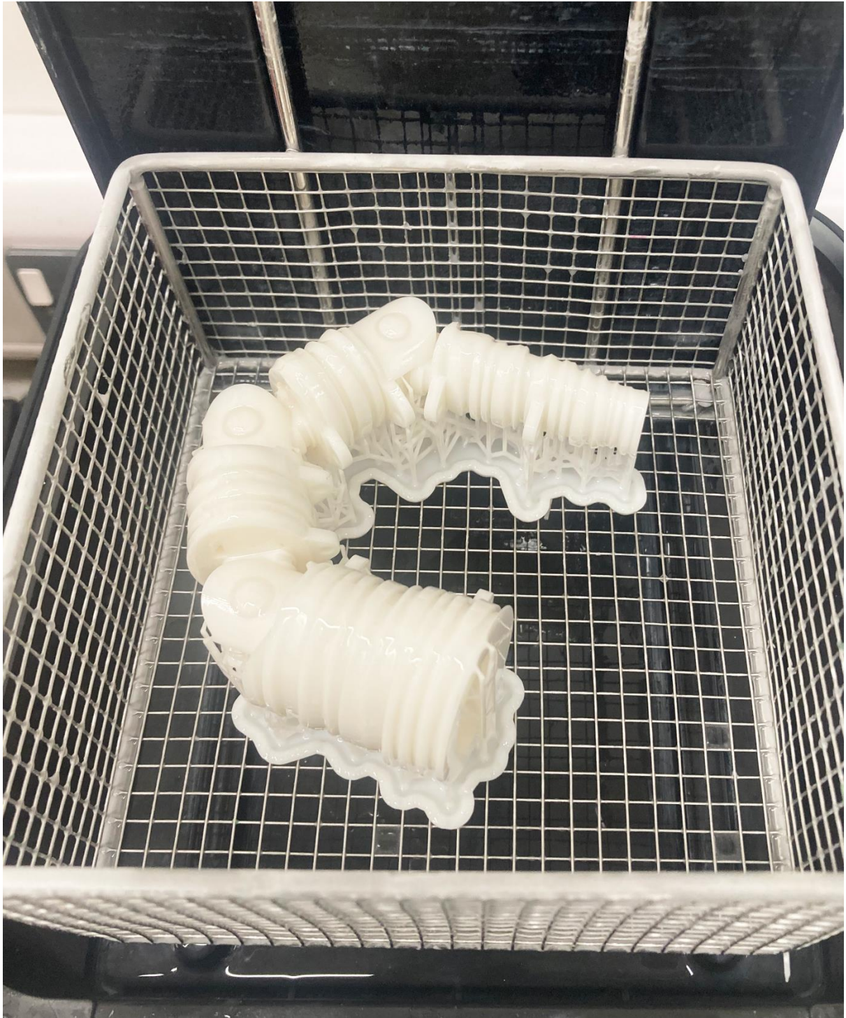
Figure 25 the complete trunk, washed out to remove the uncured resin
