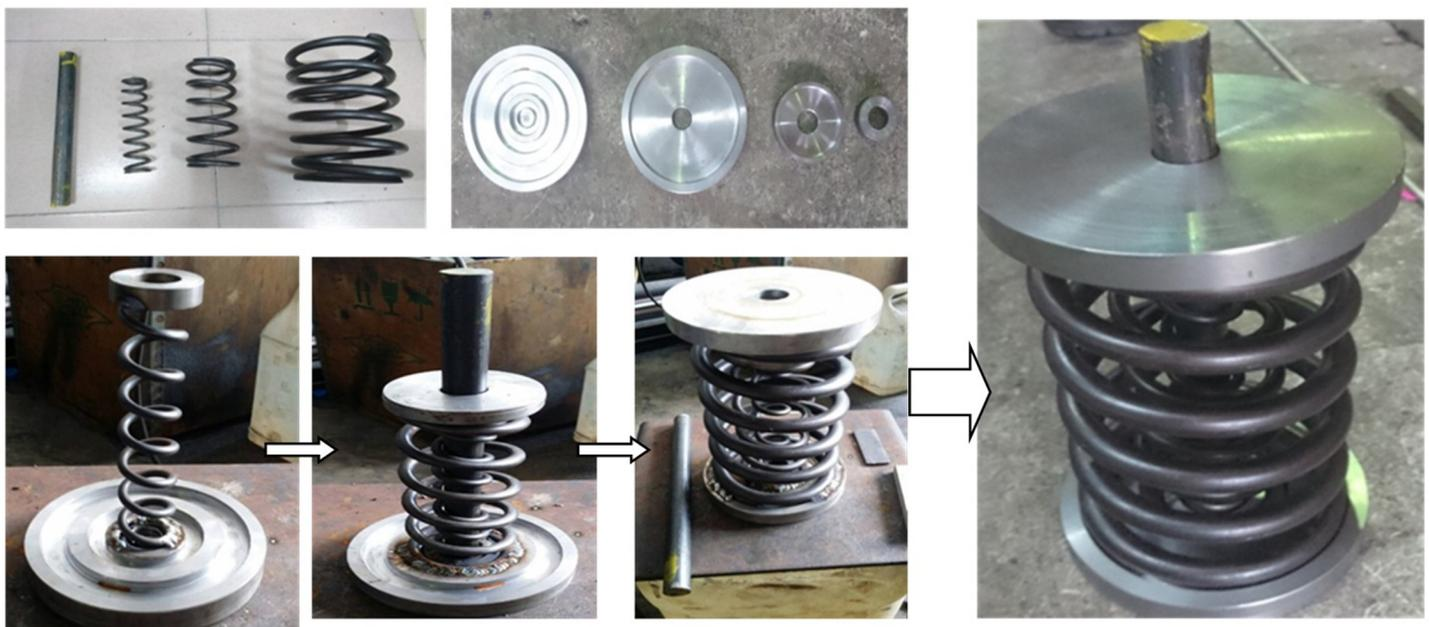
**Fig 4. The fabrication of AVSR prototype.**
