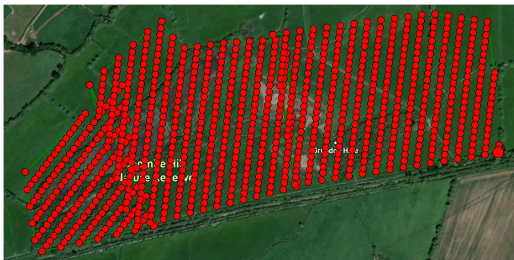
Fig 37. Flight Path and Photograph Locations for the Coombe Hill Canal and Meadows Drone Survey
