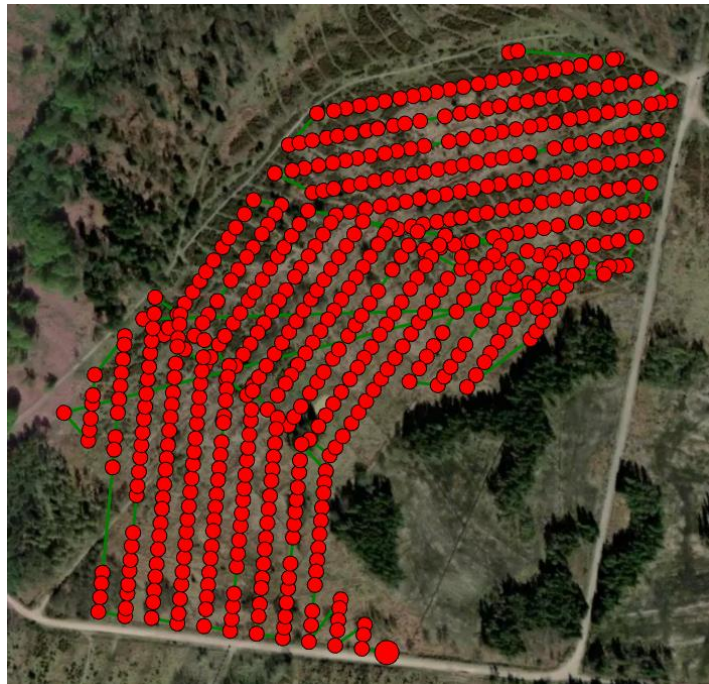
Fig 20. Flight Path and Photograph Locations for the Crabtree Hill Drone Survey
