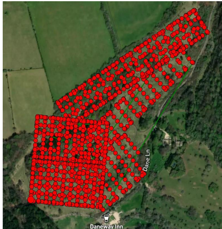
Fig 6. The Flight Path and Photograph Locations for the 2017 Daneway Banks Drone Flights
