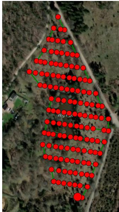
Fig 22. Flight Path and Photograph Locations for the Wigpool Drone Survey
