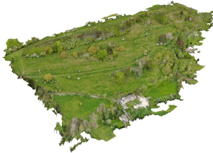
Fig 9. A 3D Model of Daneway Banks and the Surrounding Area created using a Densified Point Cloud
