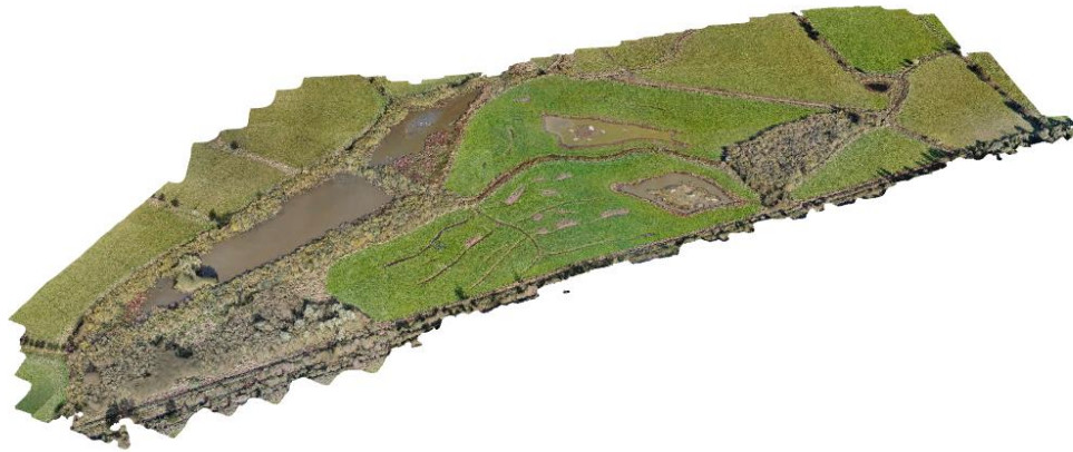
Fig 41. A 3D Model of the Study Area of Coombe Hill Canal and Meadows created using a Densified Point Cloud
