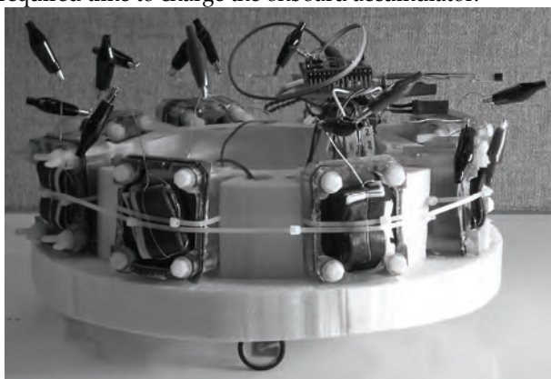
Fig. 3. EcoBot-II with O 2 MFCs onboard. Fuel cell units were placed with the open cathode facing outwards, so that the electrode could be exposed to air.
