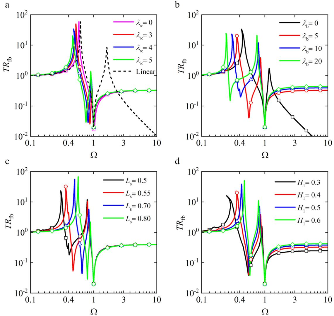
473 **Fig. 12** Force transmissibility  $TR_{fb}$  to the base under the effect of (a) stiffness ratio of the horizontal spring  $\lambda_k$ ,
