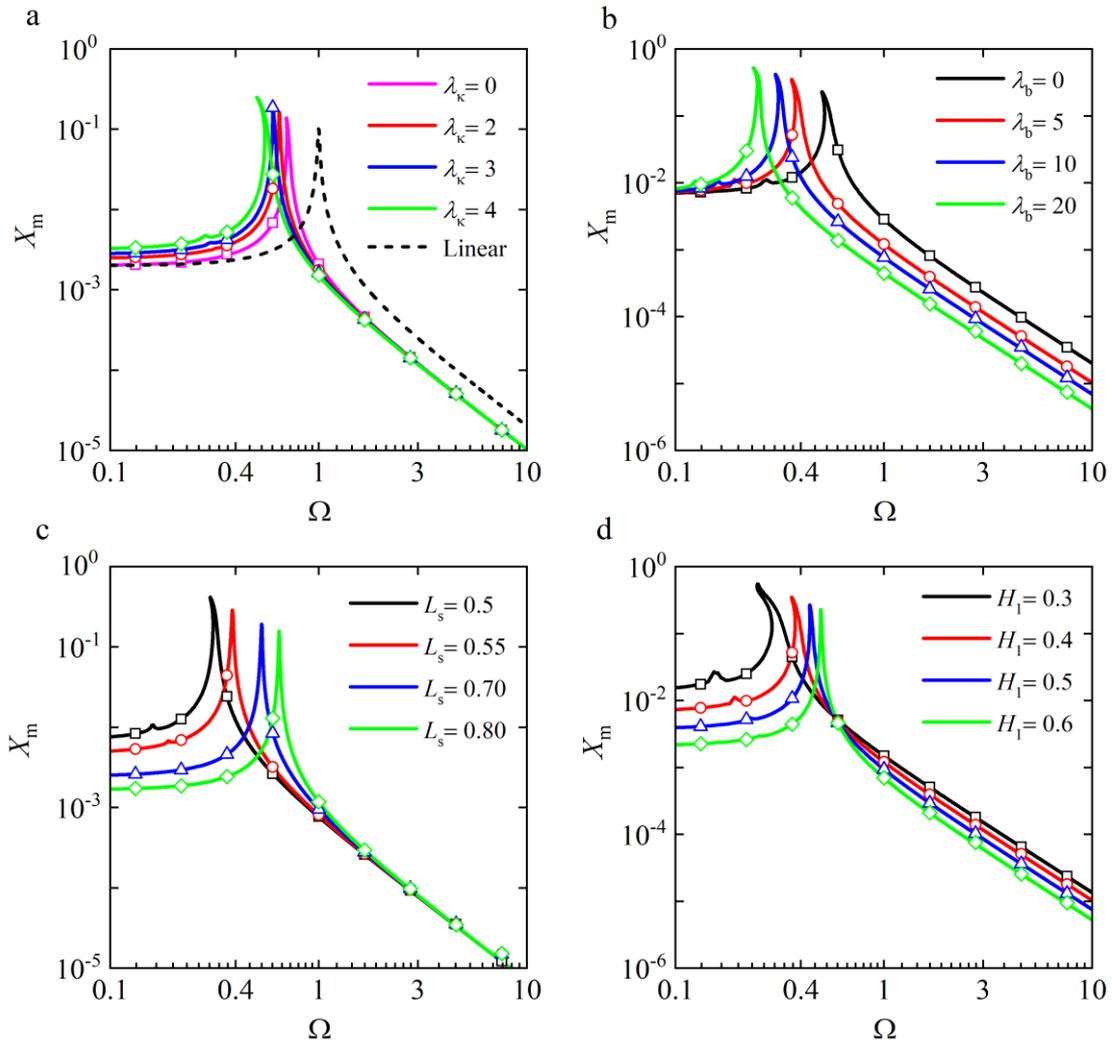
266 **Fig. 5** Maximum displacement response  $X_m$  of the equipment under the effect of (a) stiffness ratio of the horizontal
