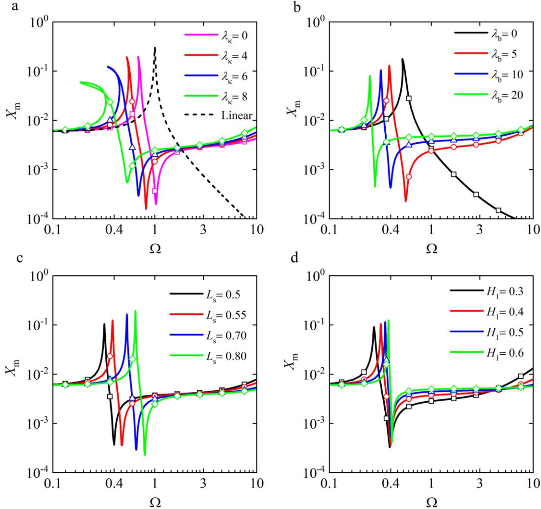
341 **Fig. 8** Maximum displacement response  $X_m$  of the equipment under the effect of (a) stiffness ratio of the
