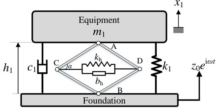
Fig. 4 Model of nonlinear isolation system with NISE under base excitation
