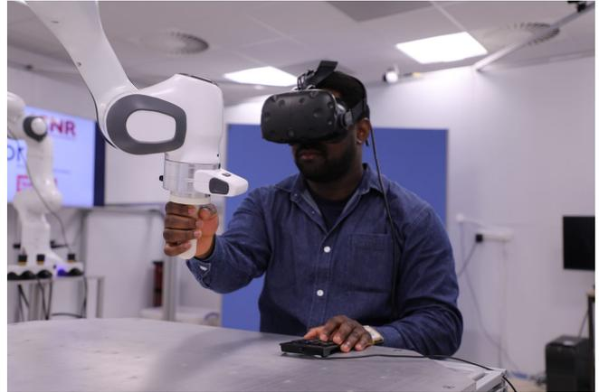
Fig. 2: The operator wearing an HTC Vive HMD and holding the teleoperation leader arm handle.
