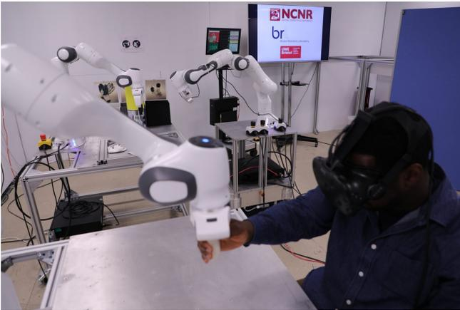
**Fig. 4:** The experiment setup, showing the operator controlling the leader arm and the camera arm in front of the remote scene controlled by the operator head movement.
