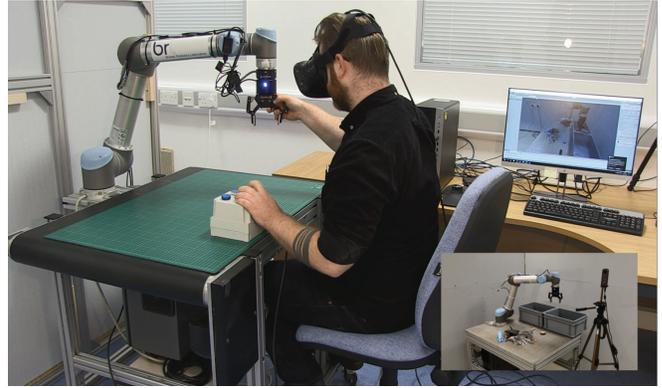
Fig. 1: Teleoperation using 360° camera video stream on HMD.
