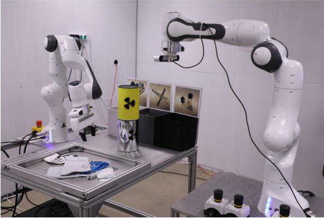
**Fig. 3:** The remote scene with the follower robot (left) and camera arm placed in front of the scene (right).
