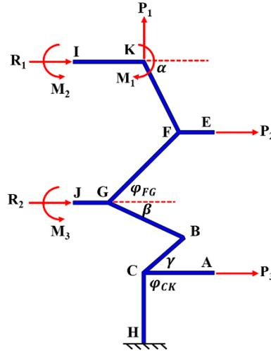
**Figure 4.** Free diagram of half of the unit cell under loading x-direction
