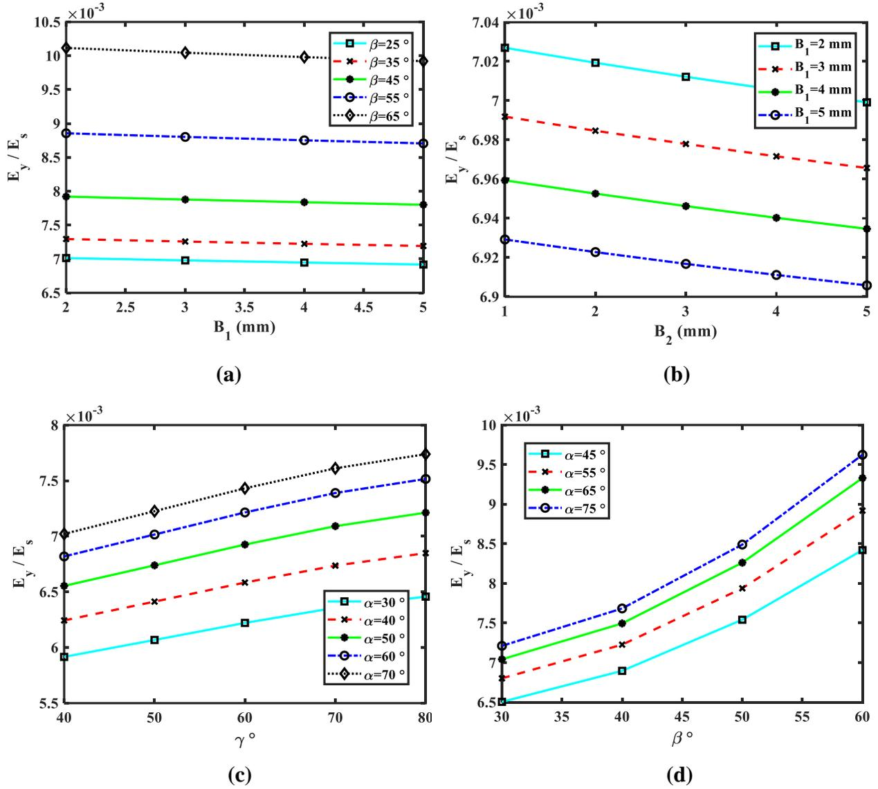
**Figure 16.** Effect of changes of a unit cell parameter on the elastic modulus in the y-direction.
