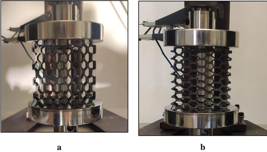
Figure 7. (a) Compression test; x-direction, (b) y-direction
