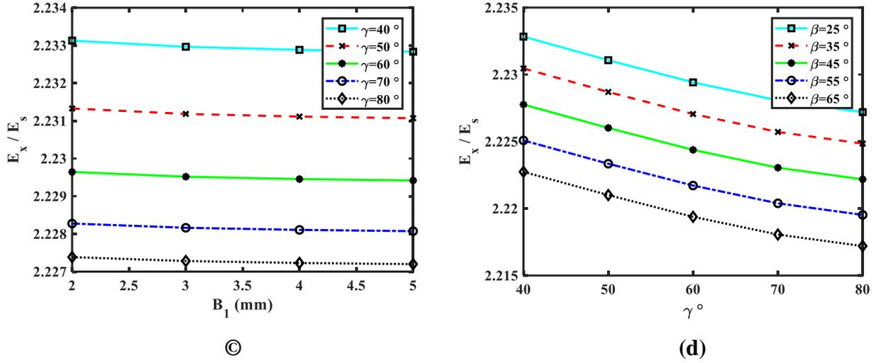
**Figure 15.** Effect of changes of a unit cell parameter on the elastic modulus in the x-direction.
