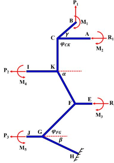
**Figure 5.** Free digram of half of the unit cell under loading y-direction
