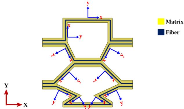
**Figure 10.** Fiber orientations in the bone-inspired unit cell
