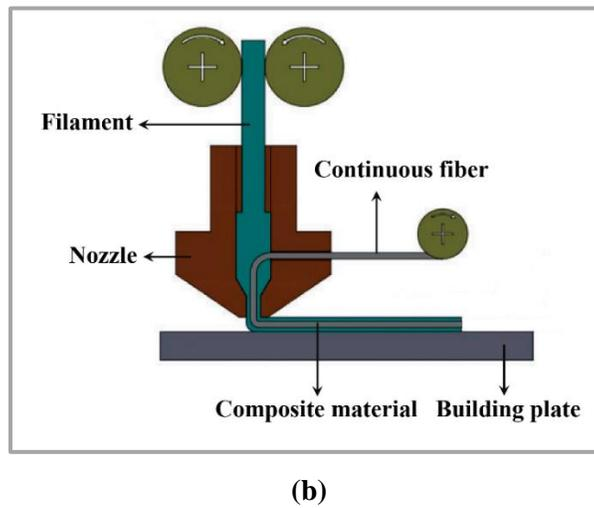
Figure 6. (a) Printing bio-inspired cellular structure with a continuous fiber, (b) Printing process[37]
