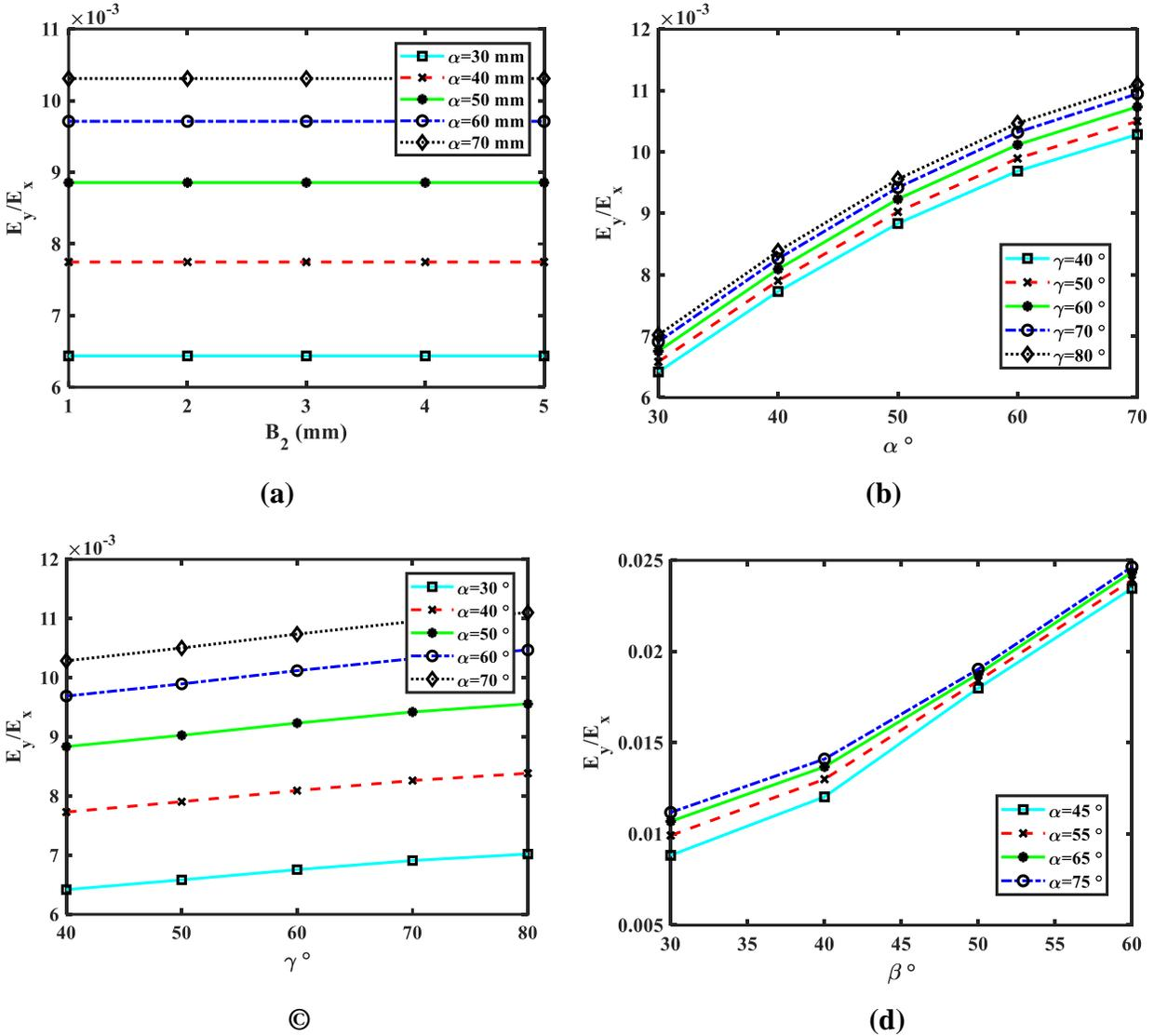
**Figure 17.** Effect of changes of a unit cell parameter on the elastic modulus in the y/x direction.
