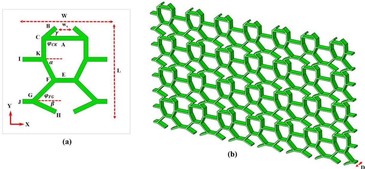
**Figure 2.** (a) The bone inspired unit cell with geometrical parameters and (b) a bone-inspired cellular structure.
