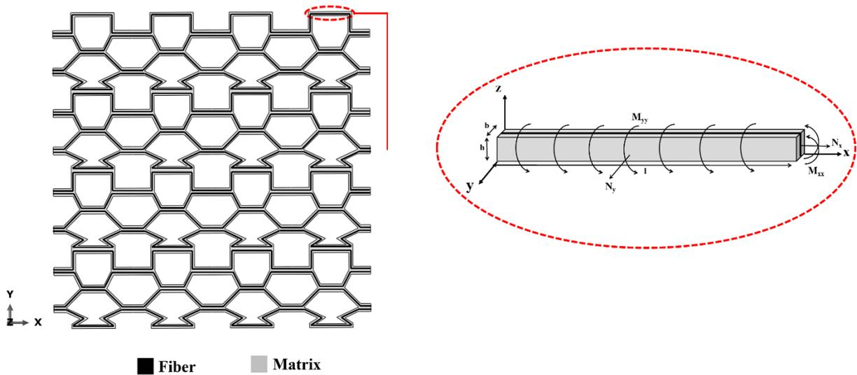
**Figure 3.** Forces and moments resultants in an orthotropic ply
