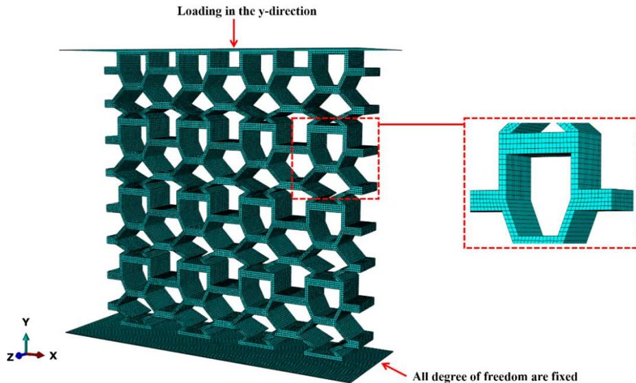
**Figure 11.** Boundary condition applied in numerical simulation
