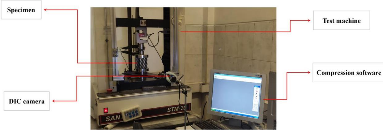
Figure 8. compression test machine with DIC camera
