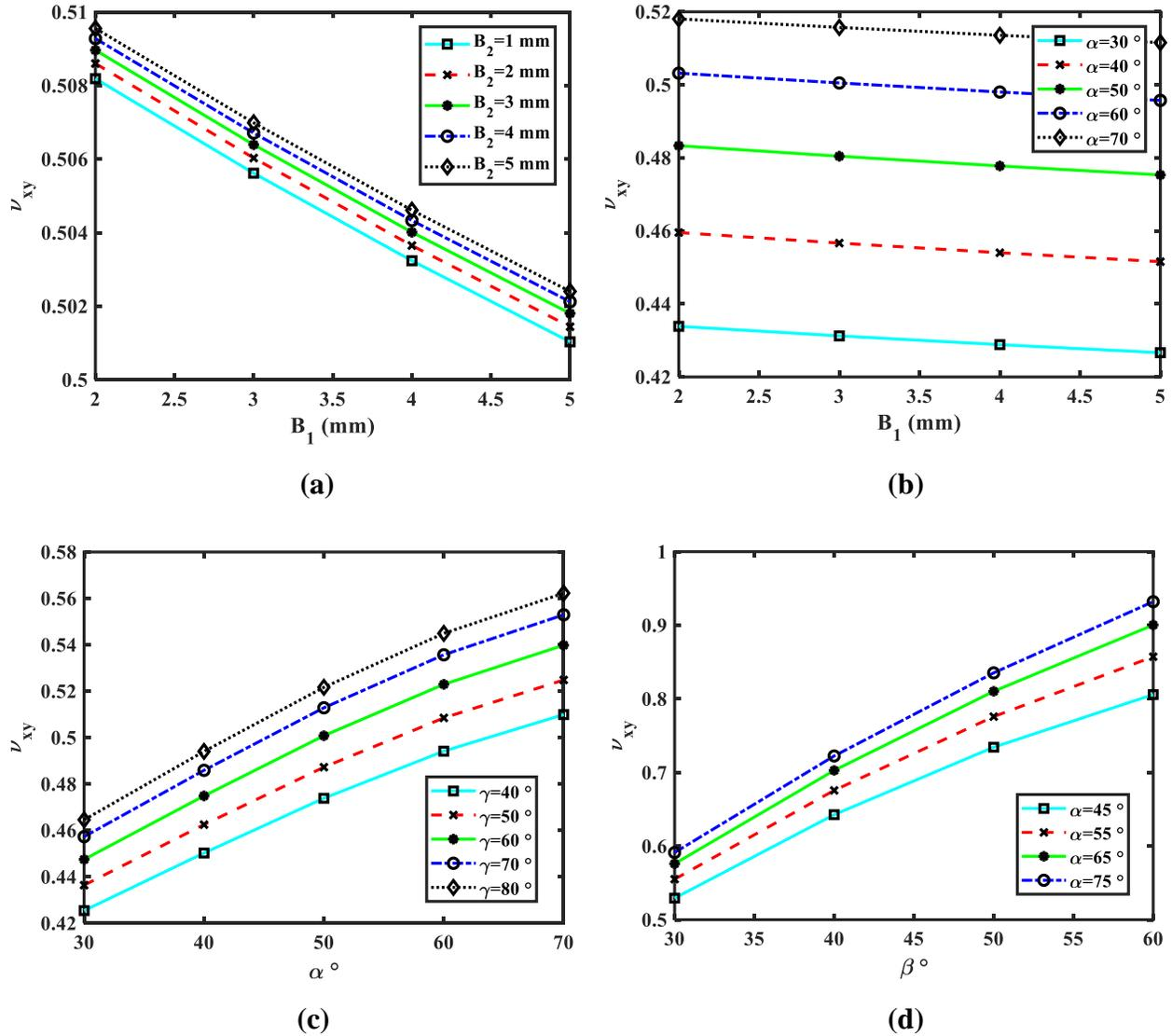
**Figure 18.** Effect of changes of a unit cell parameter on the Poisson's ratio.
