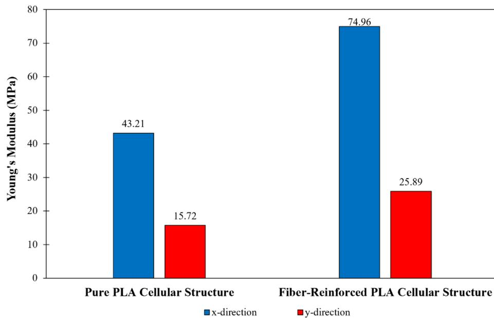
**Figure 14.** Effect of fiber in elastic properties in x and y directions
