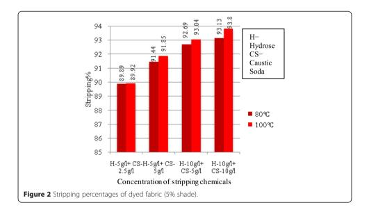
trends were found for 5% shade. Using 10 g/l hydrose and 10 g/l caustic soda and stripping at 100°C, the maximum stripping for 2.5% and 5% shades were found 92.8422% and 93.801%, respectively.
