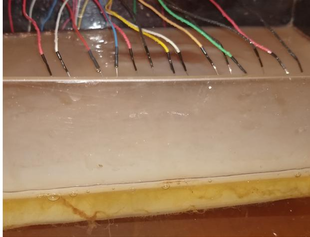
Figure 1: Experimental setup: pairs of differential electrodes are inserted into kombucha mat. The differential pairs from the left to right are (1,2), (3,4),..., (15, 16). In each pair of electrodes potential difference is measured between odd and even electrodes in the pair.
