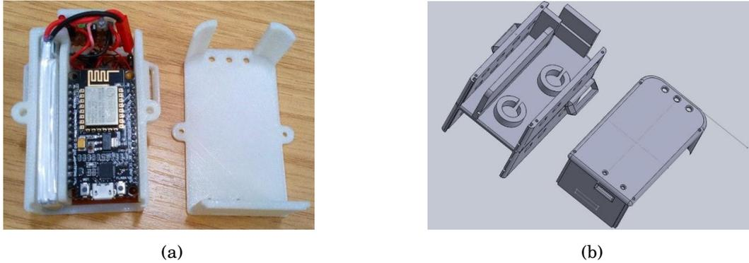
Figure 3.5: Phase-3 Haptic feedback device, (a) complete design (b) CAD design for the casing
