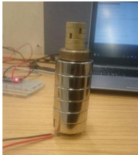
Figure 4.3: Weights placed on the FSR
