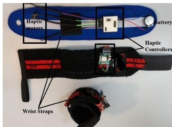
Figure 5.1: WI-FI enabled haptic feedback device
