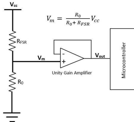
Figure 4.1: Schematic diagram of the FSR circuit
