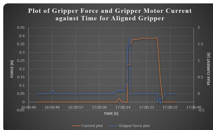
Figure 4.8: Determining optimal grasp force for a correctly aligned gripper
