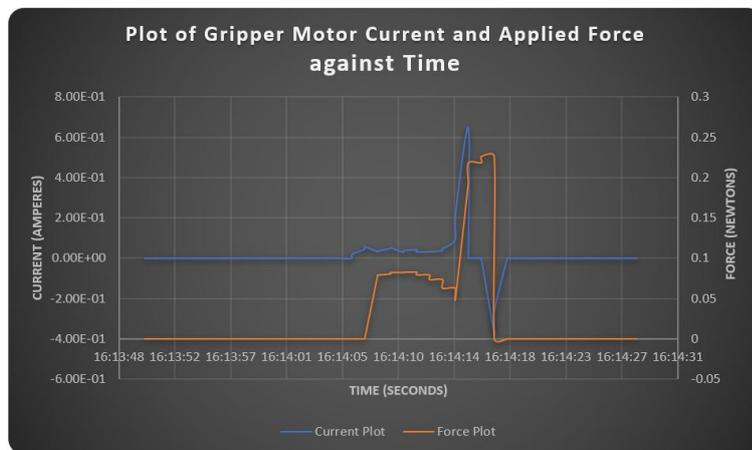
Figure 4.7: Determining optimal grasp force by plotting gripper grasp force and motor currents against time
