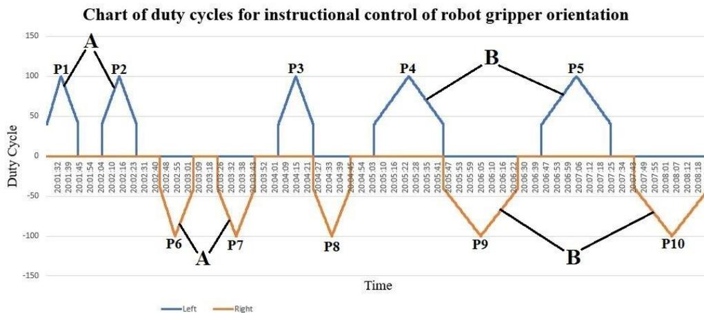
Figure 5.35: Duty cycle plot for instructional control of the robot gripper orientation
