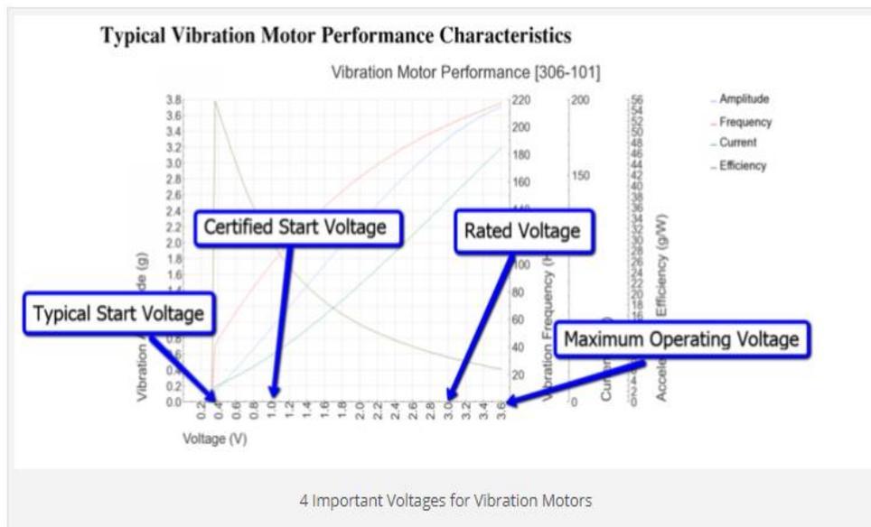
Figure 3.13: Vibrating motor voltages [148]
