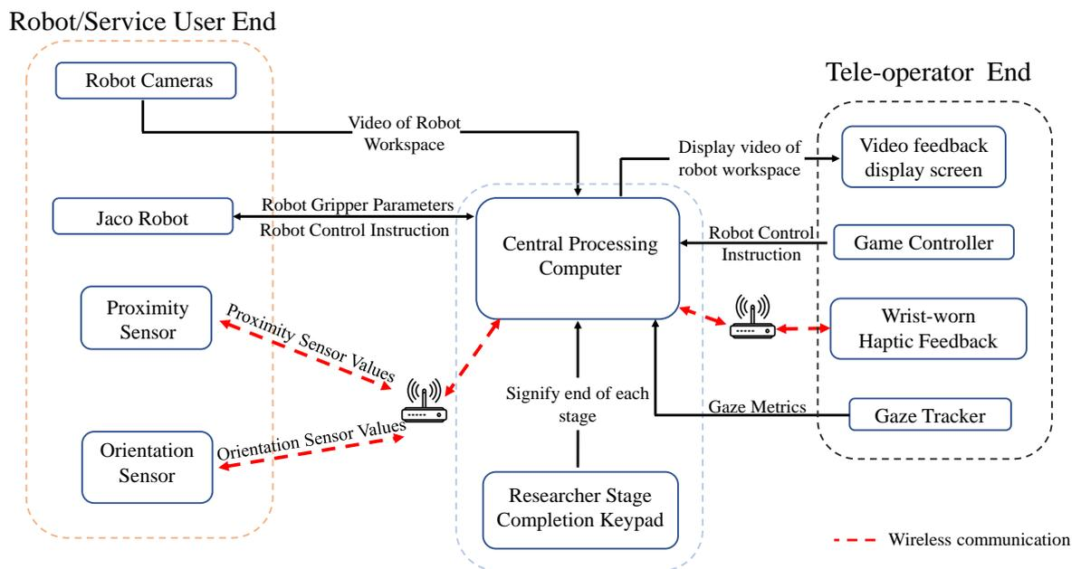
Figure 6.2: Block Diagram showing hardware and software interactions
