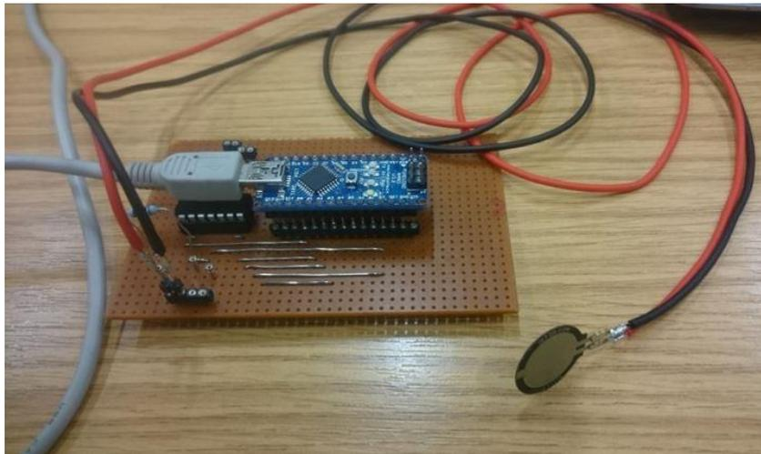
Figure 4.2: FSR and microcontroller circuit
