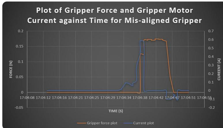
Figure 4.9: Determining optimal grasp force for a wrongly wrongly-aligned gripper
