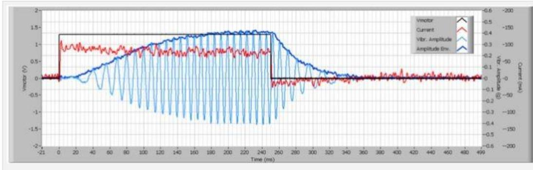
Figure 3.12: Motor voltage, amplitude, and frequency [148]
