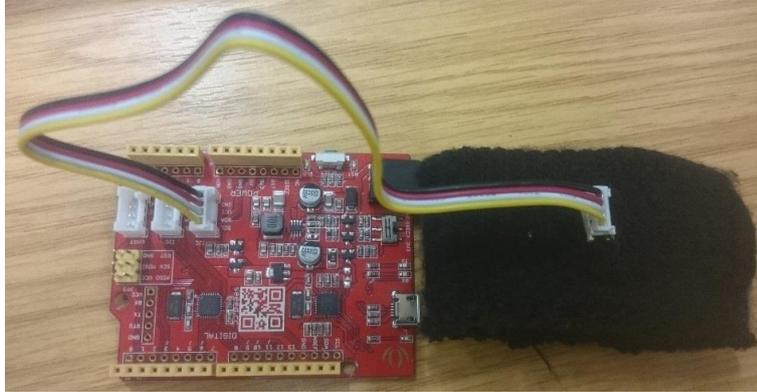
Figure 3.3: Haptic device in a wrist band with the Seeduino board
