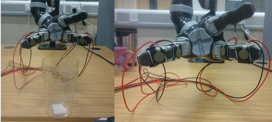
Figure 4.6: FSRs setup on the robot gripper
