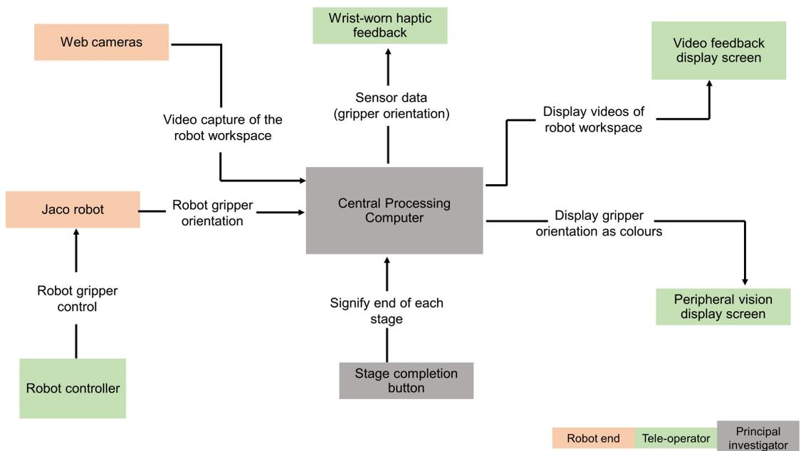
Figure 4.22: Block diagram for the study hardware and software interaction setup
