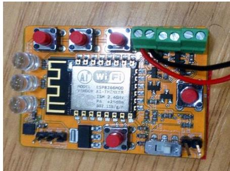
Figure 3.6: Phase-4 Haptic feedback device
