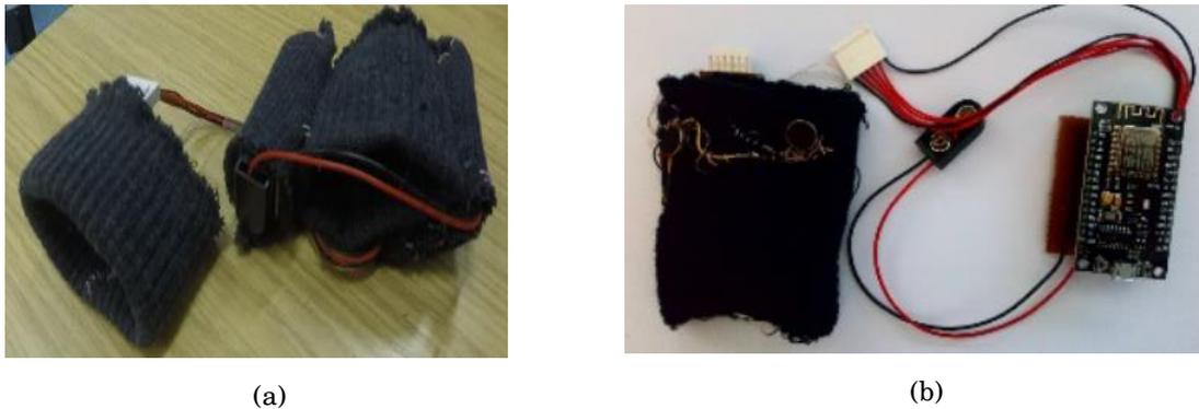
Figure 4.12: Phase-2 haptic feedback device, (a) complete design (b) haptic motor and control board
