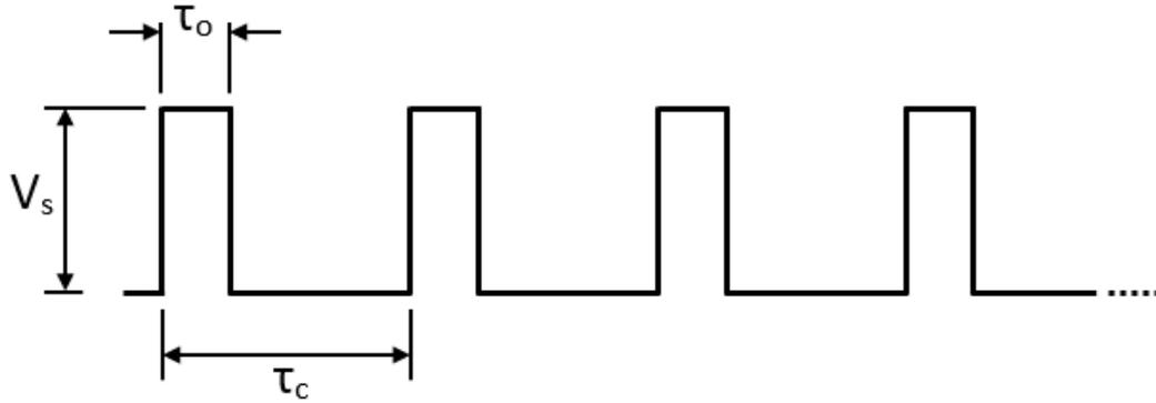
Figure 3.11: Duty cycle of pulse width modulation
