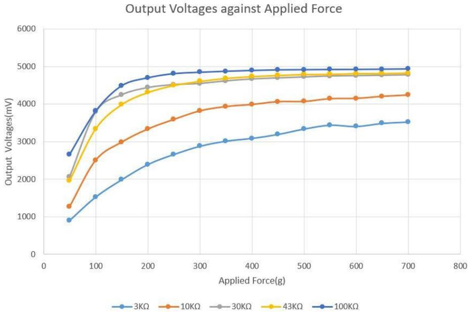
Figure 4.4: Plot of output voltages against applied force for the different known resistor values
