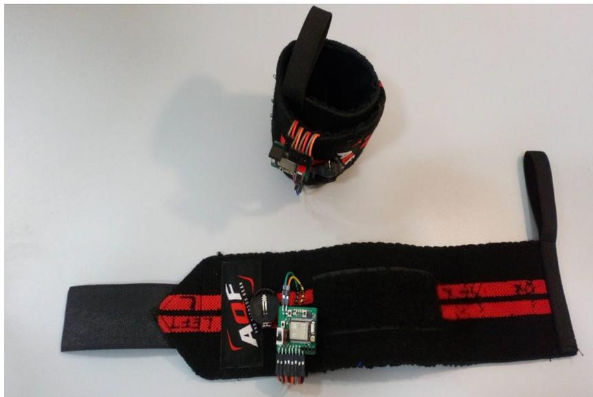
Figure 3.9: Phase 5 haptic feedback device
