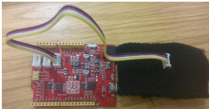
Figure 4.11: Wrist-worn haptic feedback device powered with the Seeduino board
