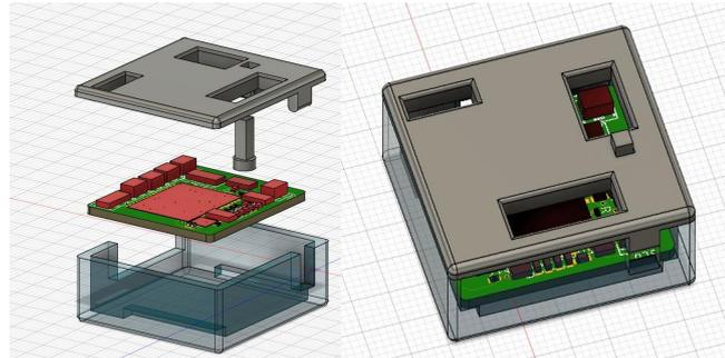
Figure 3.8: 3D model of the phase-5 haptic feedback circuitry
