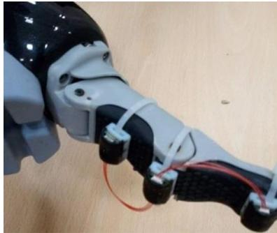
Figure 3.15: Force sensor mounted on the Jaco<sup>2</sup> robot gripper
