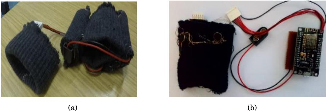
Figure 3.4: Phase-2 haptic feedback device, (a) complete design (b) haptic motor and control board
