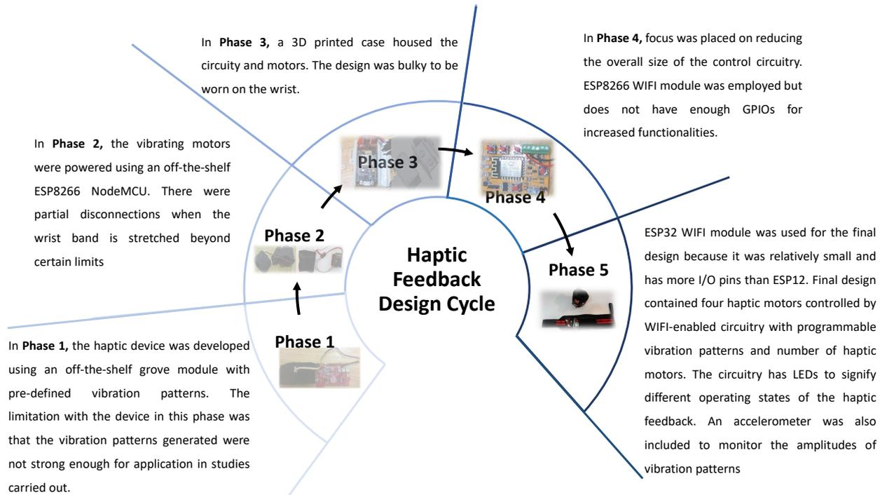
Figure 3.10: Haptic feedback design iterations
