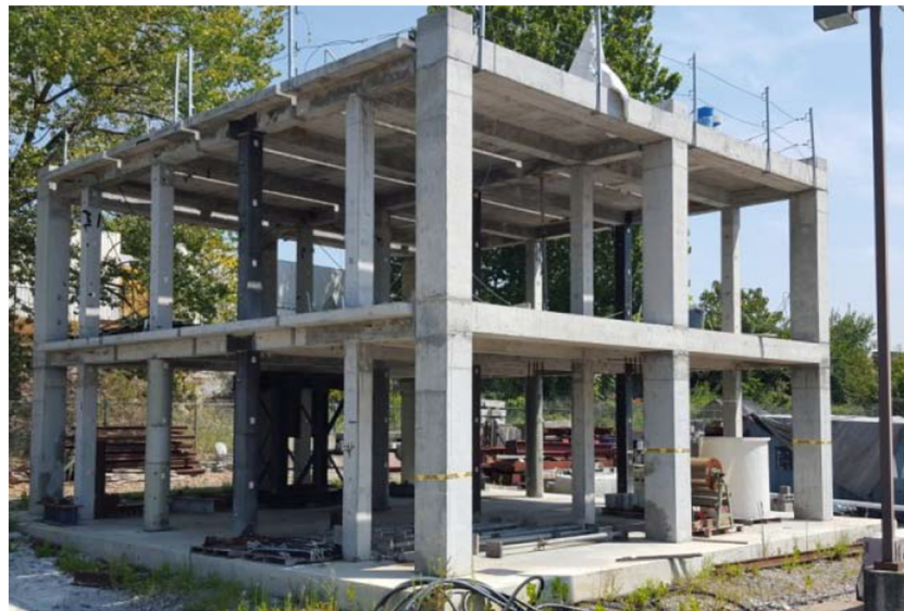
FIGURE 47 Four identical two-story, two-bay frames [29]
