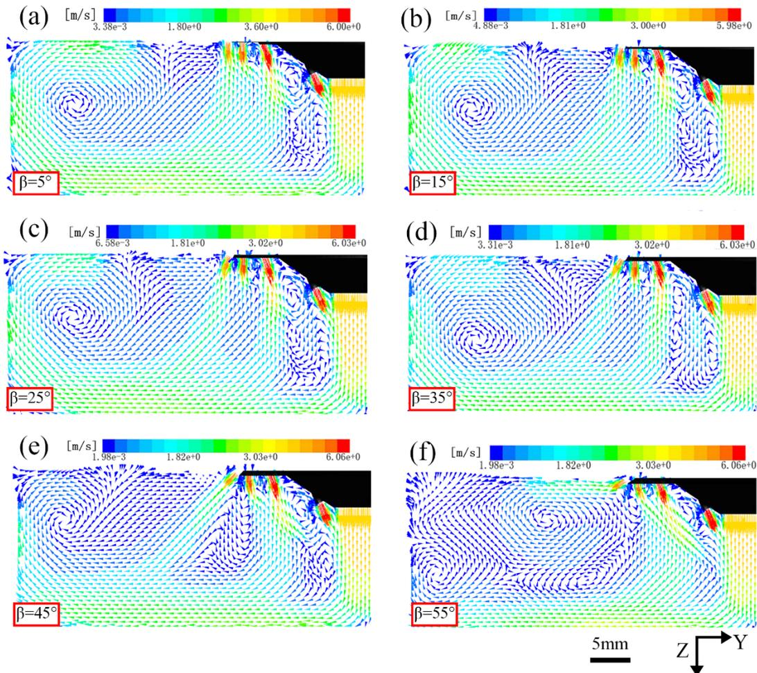
1 **Figure 11.** The simulation results of side section of velocity under different TACS flared angle
