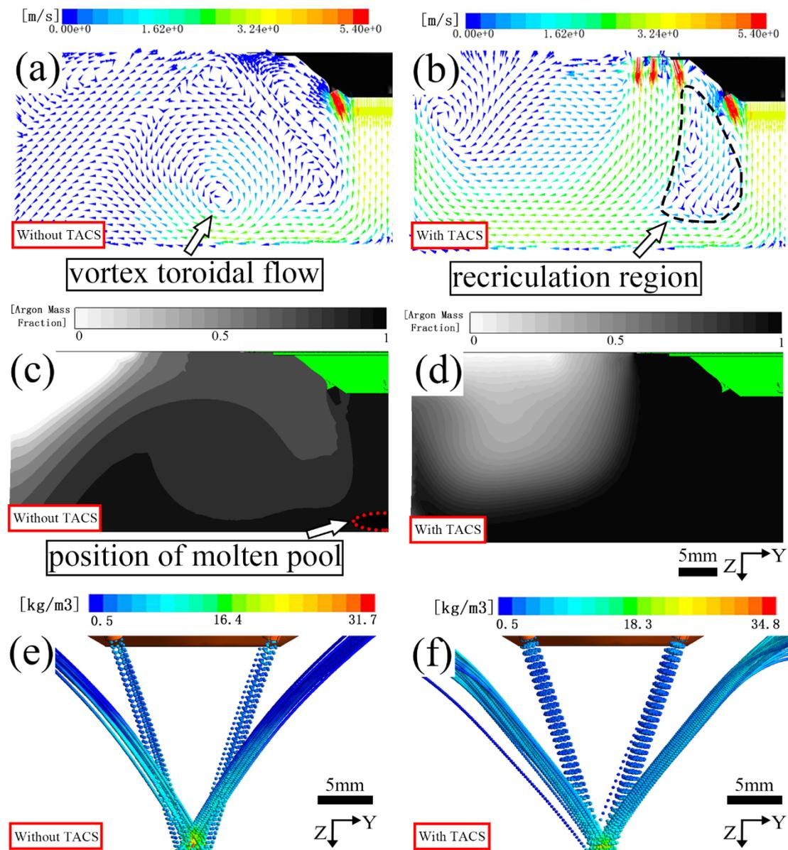
1 **Figure 8.** The simulation results of side section of velocity field, argon distribution and powder
