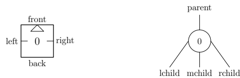
Fig. 3. A robot and its graphical node counterpart. The hinge joint is on the left-right axis.
