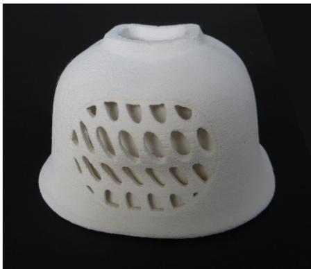
Figure 26. First fired piece showing distortion due to the firing process.
