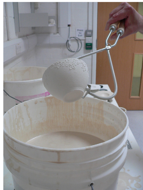
Figure 9. Dipping the sugar bowl in porcelain slip.
