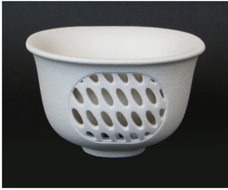
Figure 30. Peter Ting Bristol teacup coated in porcelain slip and re-fired.
