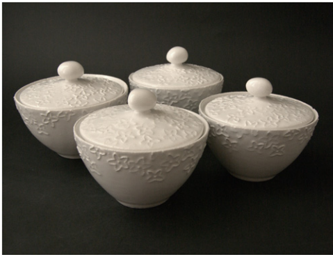
Figure 11. 3D printed ceramic sugar bowls, fired and glazed.
