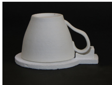
Figure 15. 3D printed cup on setter following firing.
