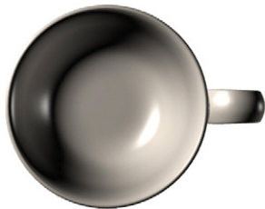
Figure 11. 3D printed ceramic sugar bowls, fired and glazed.
