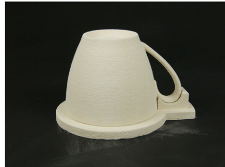
Figure 14. 3D printed cup on setter prior to firing.
