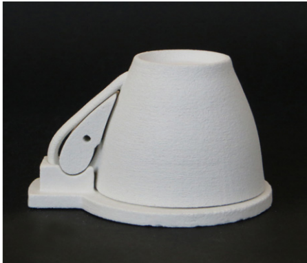
Figure 17. Cup and setter with handle support following firing.
