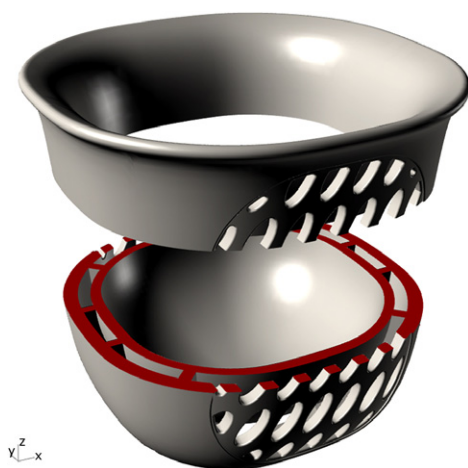
Figure 22. Cutaway drawing showing double wall design with connecting ribs.
