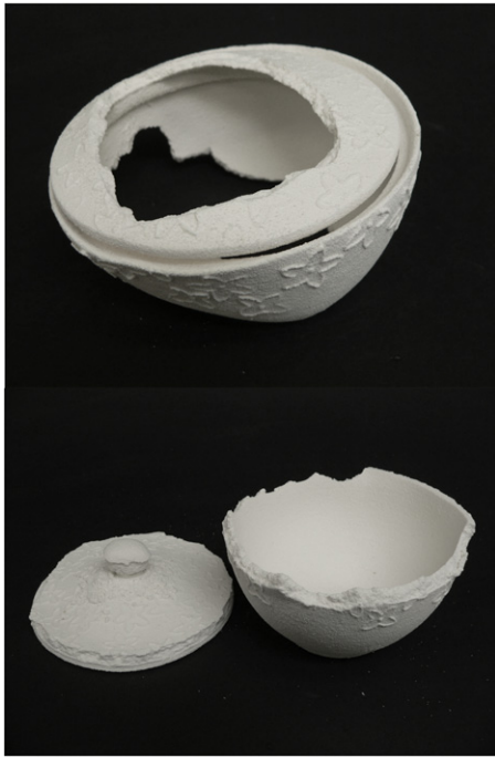
Figure 5. The first attempts at firing the 3D printed ceramic sugar bowl and lid were unsuccessful.
