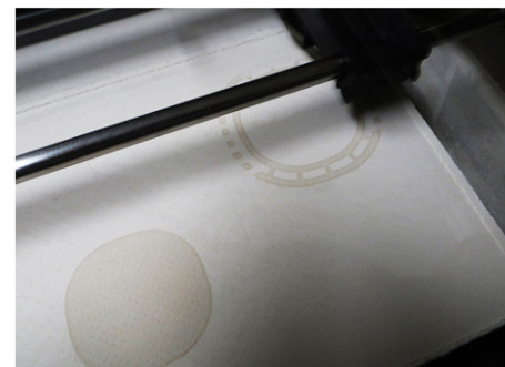
Figure 24. 3D printing teacup and support.
