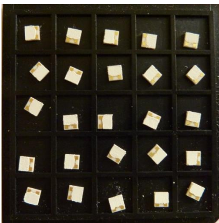
Figure 35 - Photograph of sensors coated using doctor blading method
