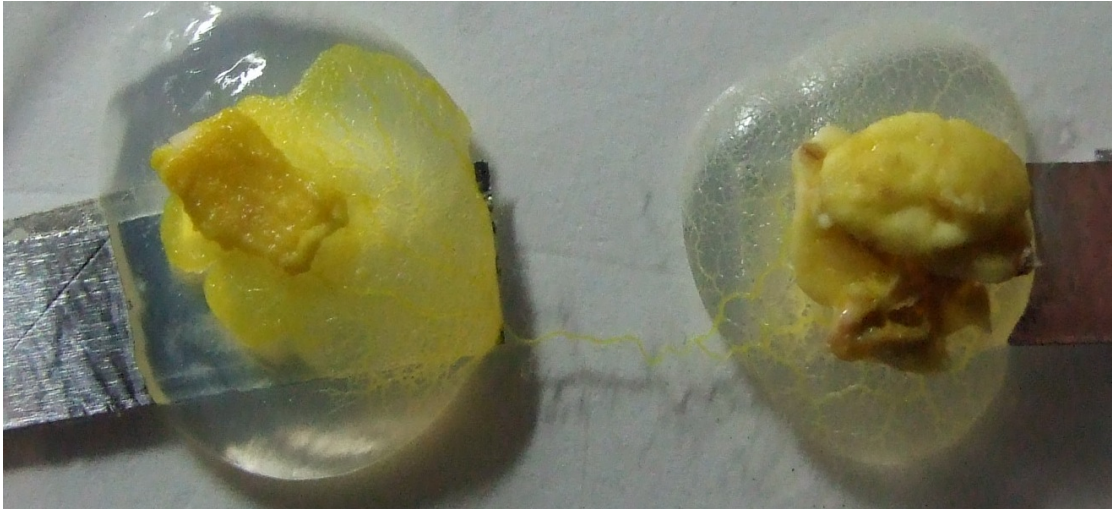
FIGURE 3.4: Photograph of a plasmodial wire spanning two agar hemispheres overlying aluminium tape electrodes. Adapted from the author's own work in Ref. [209].
